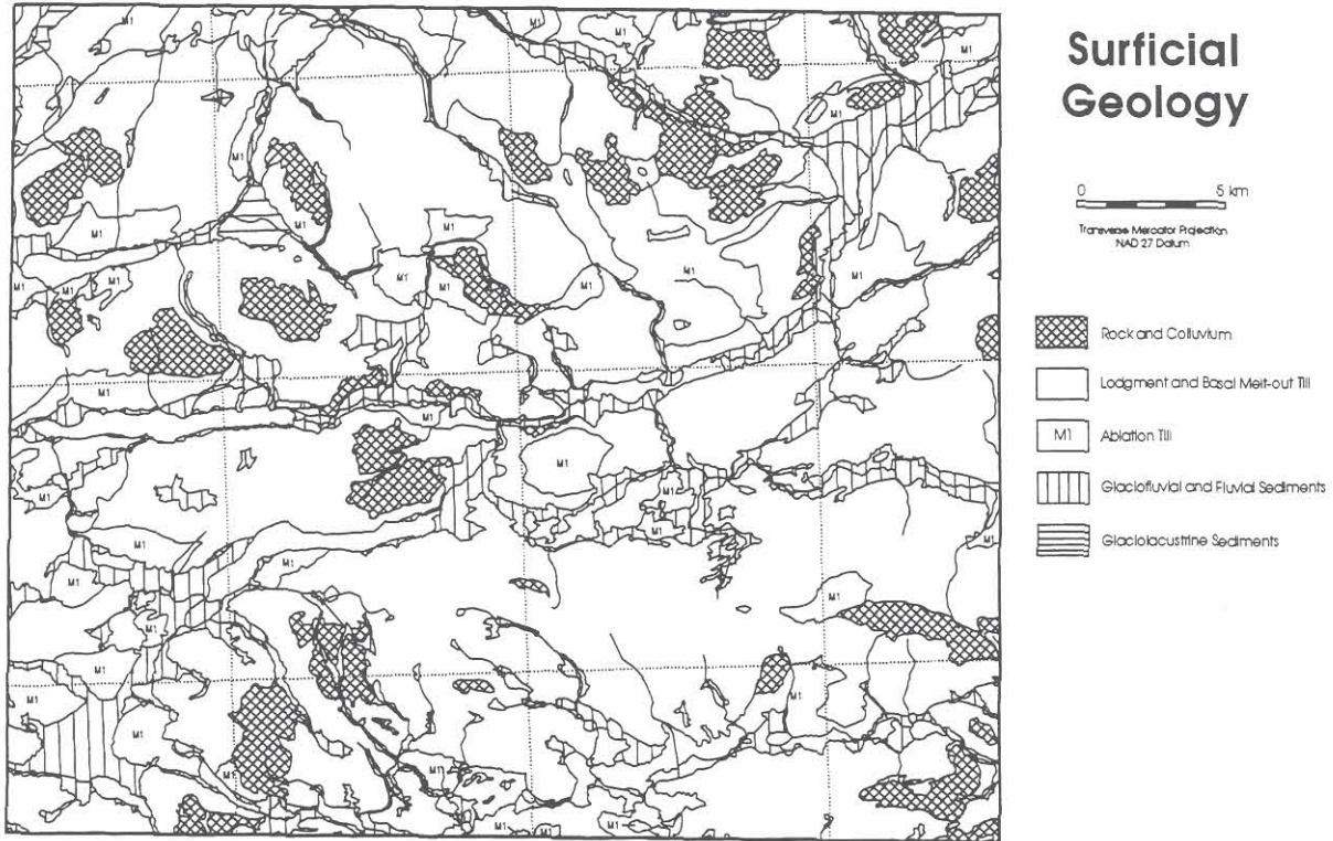
Figure 2. Surficial geology map of the Fawnie Creek map area (NTS 93 F/3). Simplified from Levson and Giles (1994). Note the dominance of morainal deposits throughout the region.
