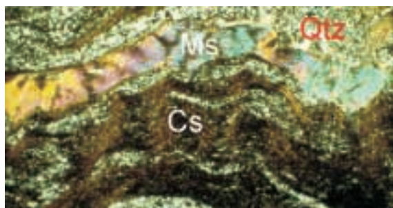
Photo 2. Photomicrograph of argillaceous partings in ribbon chert showing the development of muscovite (Ms) and crossite (Cs) layers with polygonal quartz (Qtz). A weak crenulation folds, but does not recrystallize, the authigenic minerals. The sample is number MMI97-17-4, viewed under cross polarized light. Long dimension of the photograph represents 2.5 mm.
