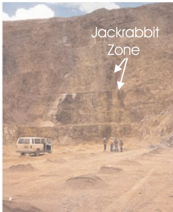
Photo 2. The Jackrabbit Zone in the south wall of the Twin Creeks megapit, Nevada. The zone consists of reddish-brown iron oxides. It is 6 to 24 metres thick, extends laterally and vertically hundreds of meters and averages 3 g/t gold, but can grade up to 34 g/t Au (Bloomstein et al. , 1991).
