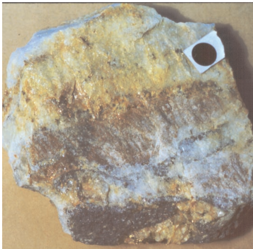
Photo 10. Molybdenite-bearing quartz stringer in granite porphyry, Trout Lake prospect (solid circle = 1 cm).
