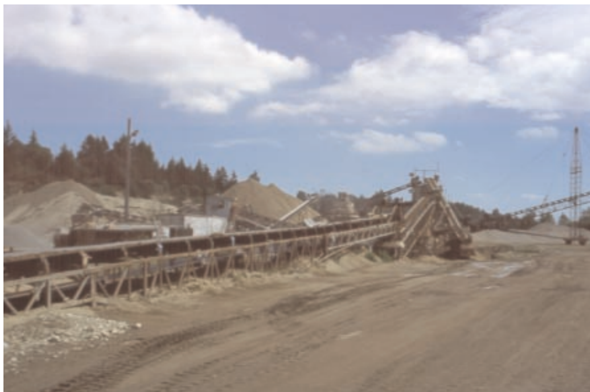
Photo 1. Gravel sizing operations - 800 meter conveyor built from jaw to crushers (Cassidy Pit).
