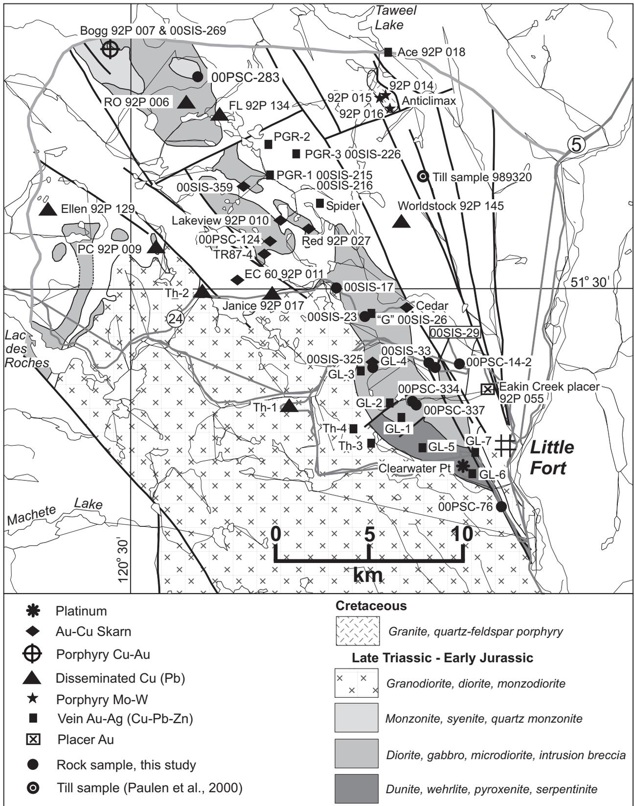
Figure 4. Locations of some of the precious and base metal mineral occurrences in the Nehalliston Plateau. Base map is derived from Figure 2, with only plutonic rocks and faults shown. The occurrences are discussed in the text.
