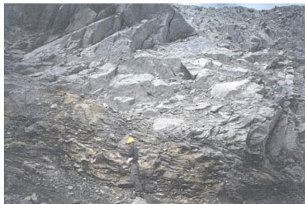
Photo 10. Sub-horizontal carbonate altered and quartz-carbonate veined shear zone cross cutting sheeted veinlets. 2870 foot bench, west wall Gibraltar East pit.
