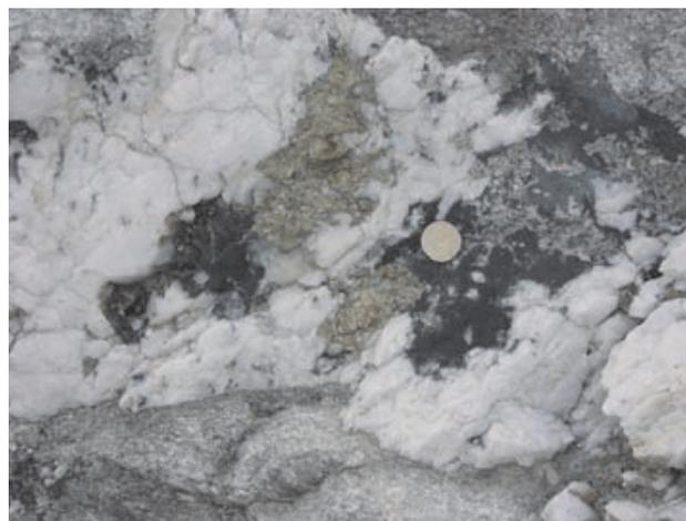
Photo 9 Detail of coarse-grained aggregates of chalcopyrite and chlorite in quartz vein shown in sub-horizontal shear zone. 3320 foot bench level, west wall Gibraltar East pit.
