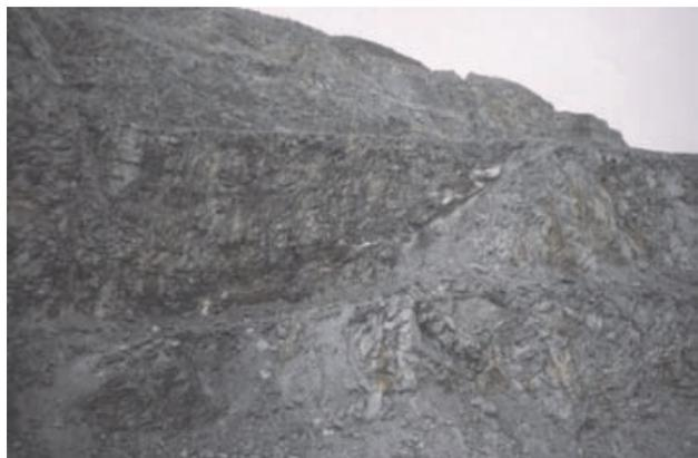
Photo 8. Discontinuous bull-white quartz vein in shallow westerly dipping shear zone between the 3150 and 3225 levels, west wall, Gibraltar East pit. Quartz veined shear zone goes from bottom left to top right.
