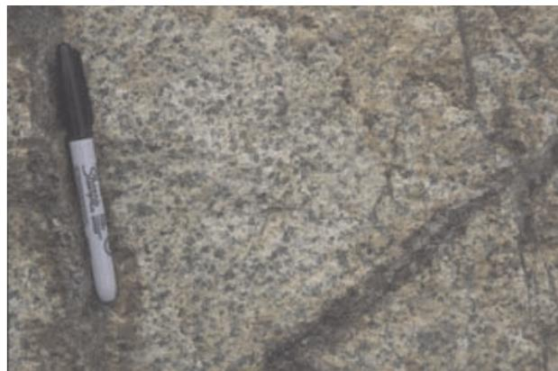
Photo 2. Typical textural character of undeformed mine phase tonalite from the west wall, Gibraltar East pit.
