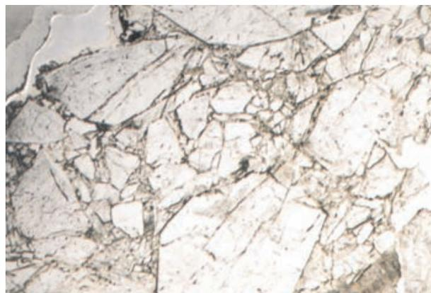
Photo 4. Quartz breccia with angular fragments of clear euhedral quartz from open vugs, Mosquito Creek deposit. Sample GR-00-73. Transmitted plane light. Width of photo 18.5 mm.
