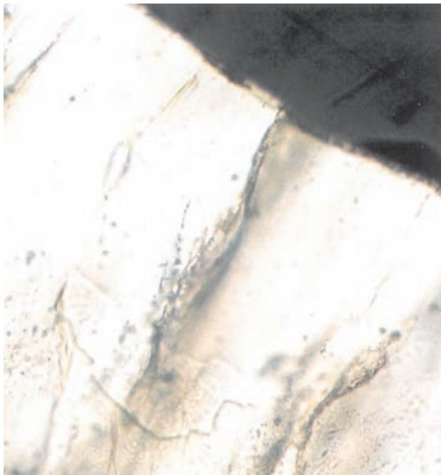
Photo 10. Recrystallized quartz zone, approximately 0.3 mm wide, around medium-grained crystalline pyrite (black) in 'massive' ore, Island Mountain deposit. Recrystallized zone comprises less than one percent tiny fluid inclusions. Sample GR-00-85. Transmitted plane light. Width of photo 340  $\mu\text{m}$ .
