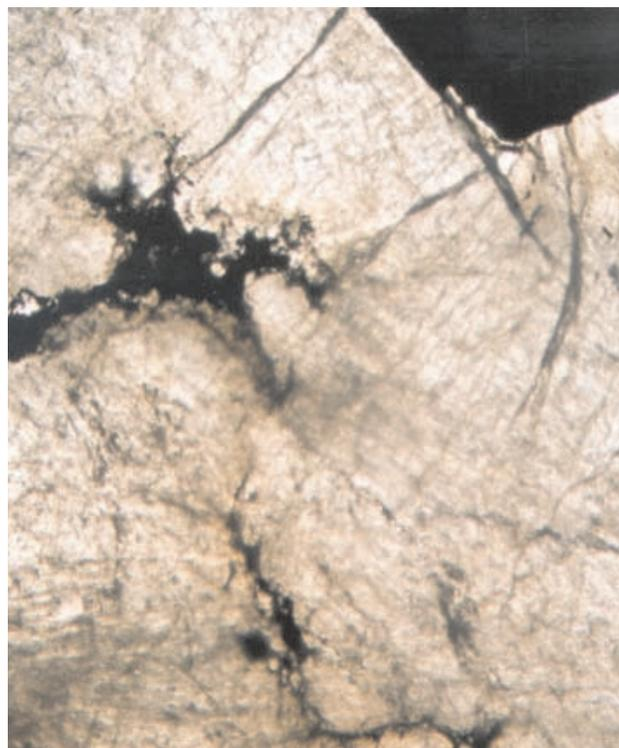
Photo 2. Abundant 'sweeping' microfractures giving appearance of wispy quartz texture in quartz-pyrite-sphalerite vein, Warspite occurrence. Note large vug left of centre. Sample GR-00-81. Transmitted plane light. Width of photo 2mm.
