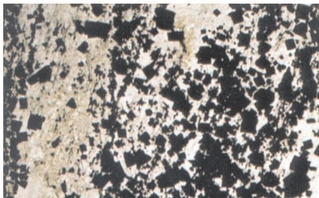
Photo 5. Medium-grained crystalline pyrite (black), quartz and minor fine-grained sericite representative of 'massive' ore, Island Mountain deposit. Sample GR-00-85. Transmitted plane light. Width of photo 18.5 mm.
