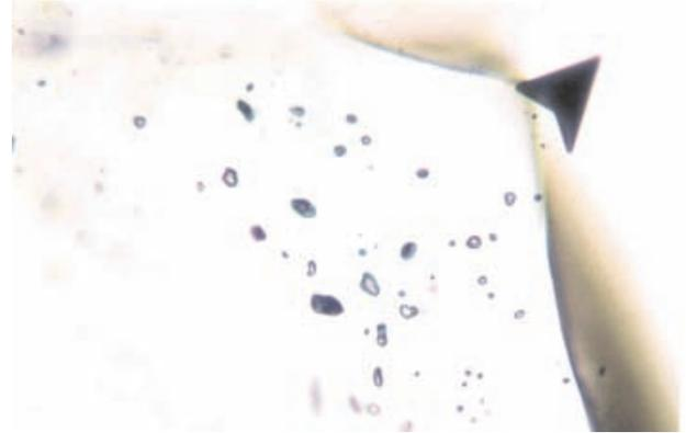
Photo 11. Pseudosecondary fluid inclusions aligned along fractures in recrystallized quartz proximal to pyrite crystals (black), 'massive' ore, Mosquito Creek deposit. Note occurrence of 2 phase liquid-rich and monophasic vapour-rich fluid inclusions trapped in the same healed fracture. This photo is an enlargement of area right of centre of Photo 9. Sample GR-00-68. Transmitted plane light. Width of photo 300  $\mu$ m.
