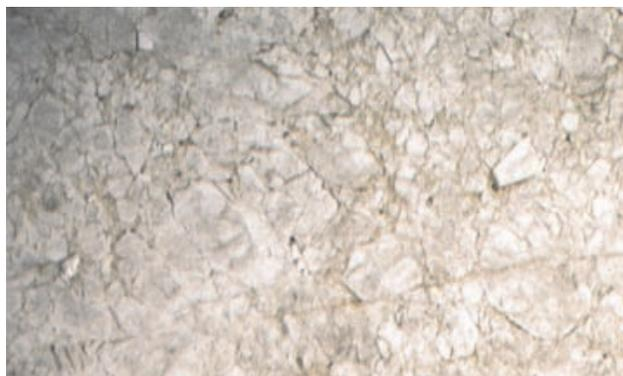
Photo 3. Quartz breccia with angular fragments from 0.5 to 2 cm provides evidence of brittle deformation near footwall of BC Vein above Bonanza Ledge. Open-space filling with clear euhedral quartz crystals is noted in this sample. Sample GR-00-46. Transmitted plane light. Width of photo 18.5 mm.
