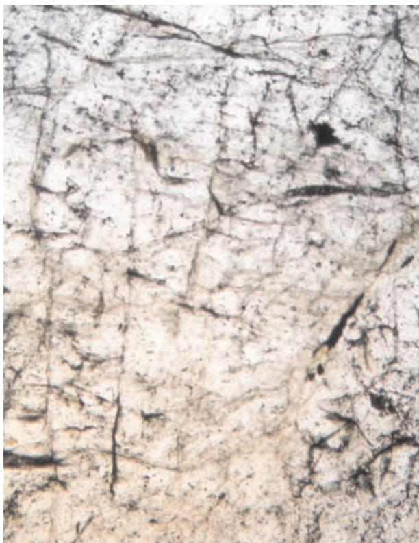
Photo 1. Highly fractured 'bull' quartz vein, Cariboo Gold Quartz deposit. Note open vug lined with quartz crystals top right of photo. Sample CGQ-FI-3. Transmitted plane light. Width of photo 2mm.
