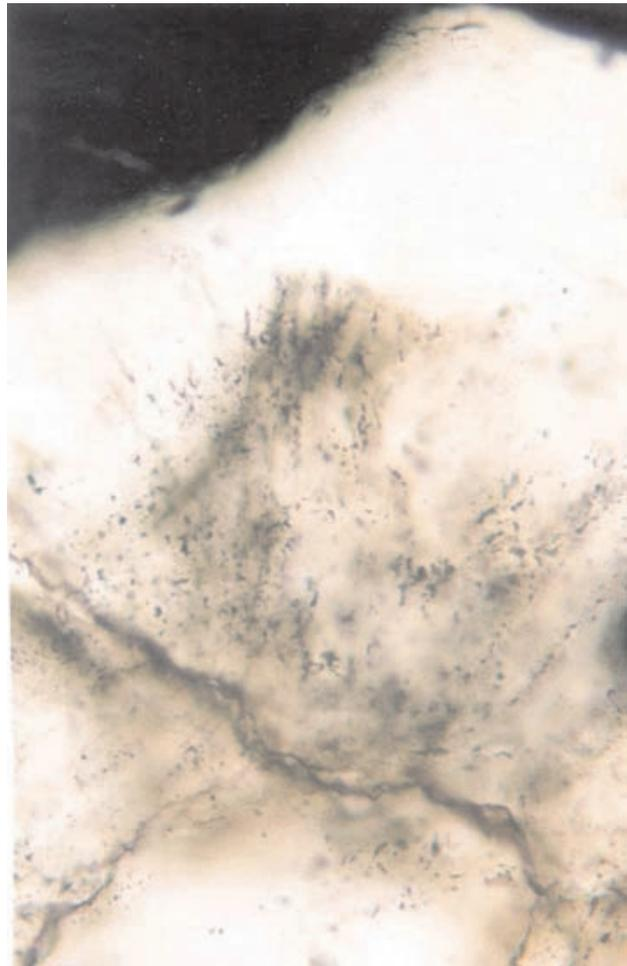
Photo 8. Tiny (<1 micrometre) primary fluid inclusions aligned along growth zones in quartz proximal to medium-grained pyrite in 'massive' ore, Mosquito Creek deposit. This photo is an enlargement of top right of Photo 7. Sample GR-00-68. Transmitted plane light. Width of photo 400 µm.
