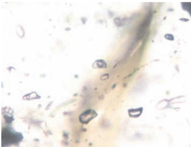
Photo 14. Coexisting monophase vapour-rich Type V inclusions and two phase liquid-rich Type IV inclusions aligned along a secondary fracture plane in quartz from a massive 'bull' quartz vein, Cariboo Gold Quartz deposit. Sample CGQ-FI-3. Transmitted plane light. Width of photo 160  $\mu\text{m}$ .
