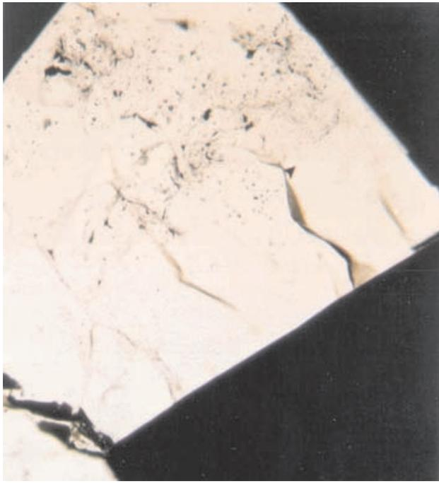
Photo 9. Recrystallized quartz zone, approximately 0.5 mm wide, with virtually no fluid inclusions, around medium-grained pyrite (black) in massive ore, Mosquito Creek deposit. Note area of enlargement for Photo 11 is right of centre of Photo 9. Sample GR-00-68. Transmitted plane light. Width of photo 2mm.
