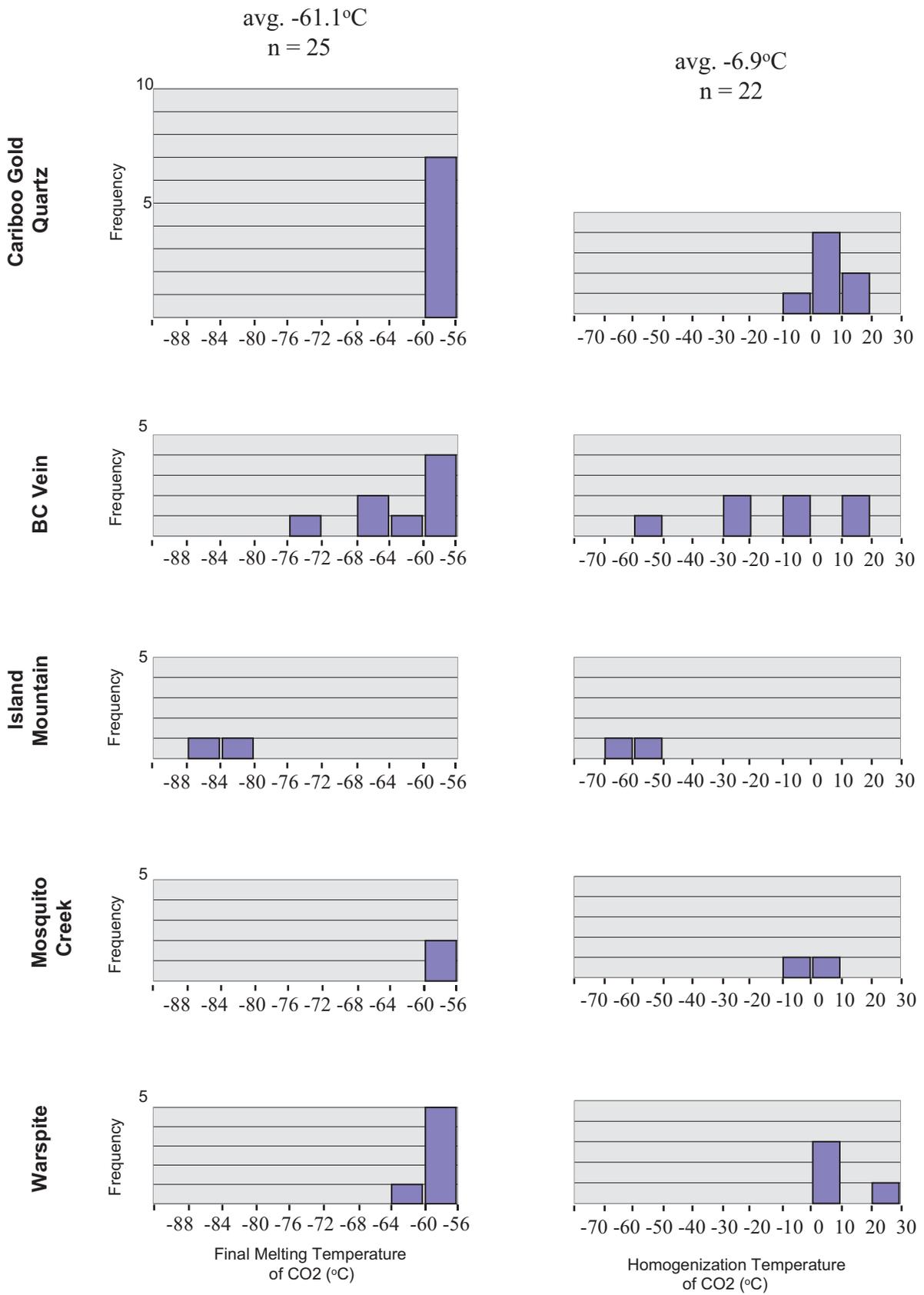
Figure 5. Temperatures of final CO<sub>2</sub> melt and CO<sub>2</sub> homogenization of Type V (CO<sub>2</sub>-CH<sub>4</sub>±N<sub>2</sub>) fluid inclusions.
