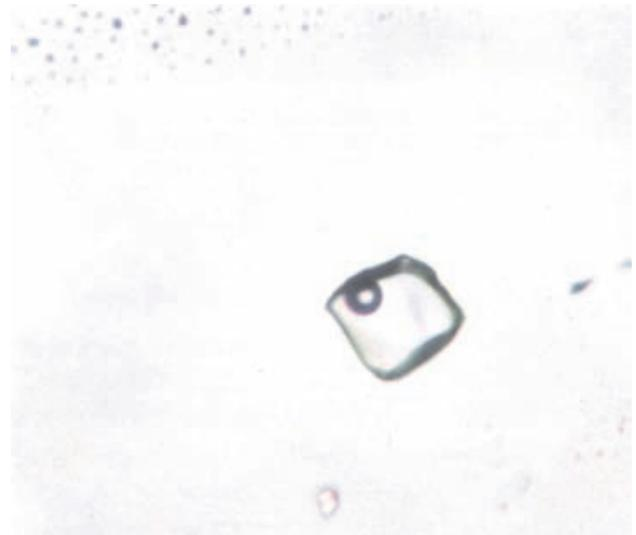
Photo 12. Negative crystal - shaped Type I fluid inclusions characterized by 2 aqueous phases: liquid and vapour in vein quartz, Mosquito Creek deposit. Sample GR-00-67. Transmitted plane light. Width of photo 160  $\mu$ m.
