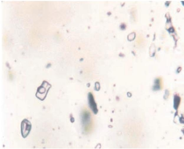
Photo 13. Smooth to negative crystal - shaped Type III fluid inclusions in a massive 'bull' quartz vein, Cariboo Gold Quartz deposit. Note solid 'daughter' crystals in the fluid inclusions left of centre and far right. Sample CGQ-FI-4. Transmitted plane light. Width of photo 160  $\mu\text{m}$ .
