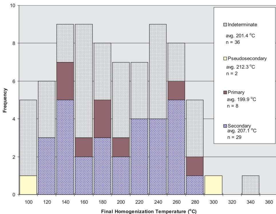
Figure 6. Distribution of primary, pseudo-secondary, secondary and indeterminate fluid inclusion origins with respect to final homogenization temperatures, to the aqueous phase, for Type I and IV fluid inclusions in quartz collected from quartz vein and massive pyrite samples from the Cariboo Gold Quartz, Island Mountain, Mosquito Creek mines and BC, Warspite and Perkins veins, respectively.
