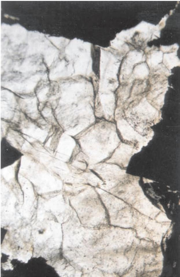
Photo 7. Subhedral to anhedral quartz crystals adjacent to medium-grained crystalline pyrite (black) in 'massive' ore, Mosquito Creek deposit. Evidence of quartz recrystallization? seen as fine-grained quartz crystals with 120°C grain boundaries at top right of photo. Note area of enlargement for Photo 8 is top right of photo 7. Sample GR-00-68. Transmitted plane light. Width of photo 2mm.
