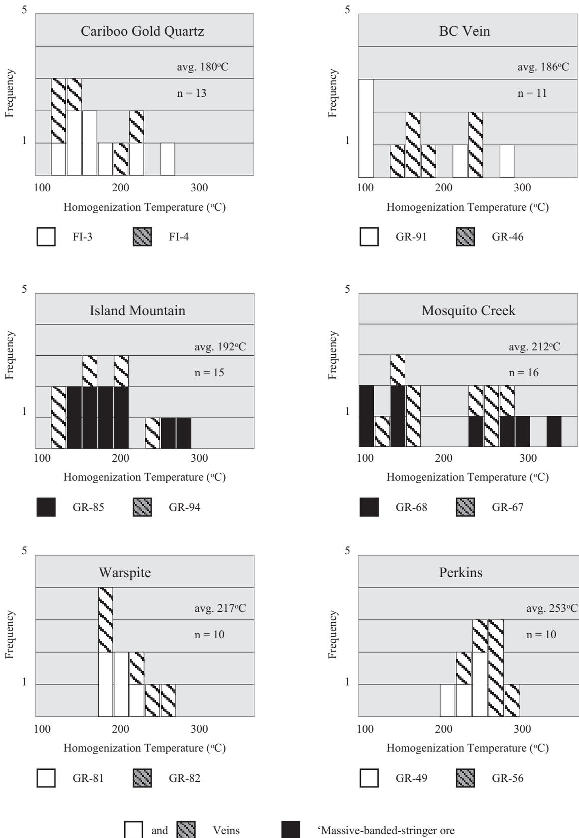
Figure 8. Final fluid inclusion homogenization temperatures (range, average and number), to the aqueous phase, for Type I and IV fluid inclusions from the Cariboo Gold Quartz, Island Mountain, Mosquito Creek mines and BC and Warspite veins, respectively. Note the diagrams share common x axes.
