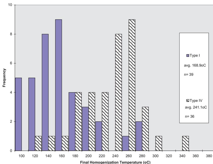
Figure 3. Type I (aqueous) versus Type IV (CO<sub>2</sub>-bearing) fluid inclusion final homogenization temperatures, to the aqueous phase, in quartz from all vein and massive pyrite samples evaluated in this study.
