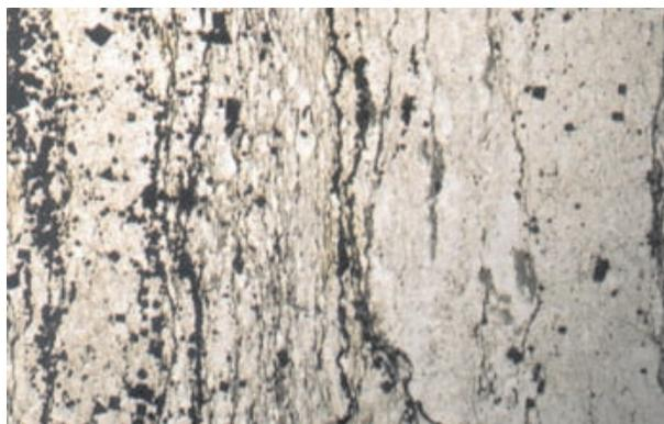
Photo 6. Fine and medium-grained crystalline pyrite (black), quartz, minor sericite and carbonate representative of 'banded' ore, Island Mountain deposit. Sample GR-00-88. Transmitted plane light. Width of photo 18.5 mm.
