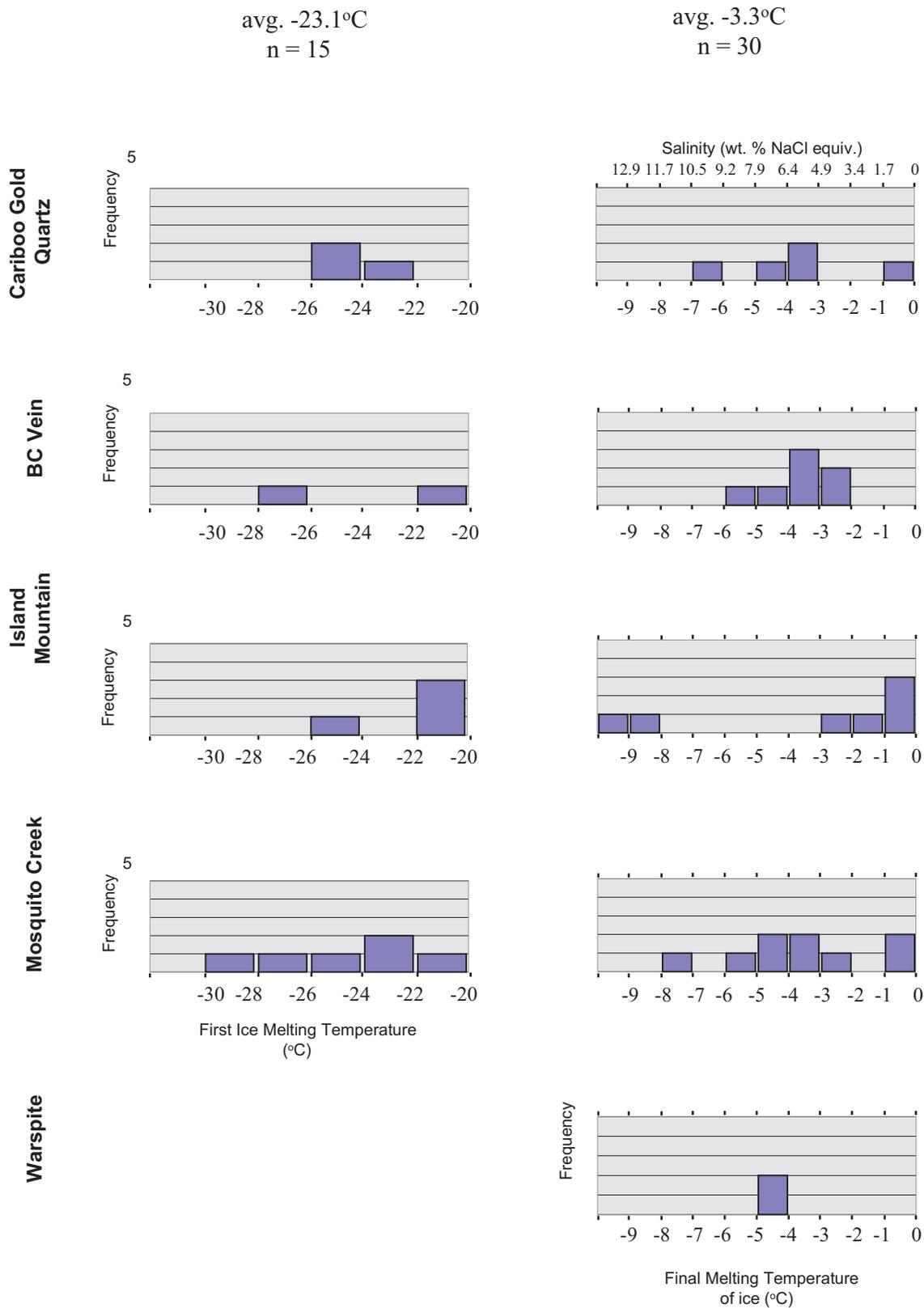
Figure 2. Temperatures of first melt and final melt of Type I (aqueous) fluid inclusions from the Cariboo Gold Quartz, Island Mountain, Mosquito Creek mines and BC and Warspite veins, respectively. The first melt approximates the eutectic temperatures of the fluid inclusions. The final melt is used to calculate the equivalent salinity. Note the diagrams share common x axes.
