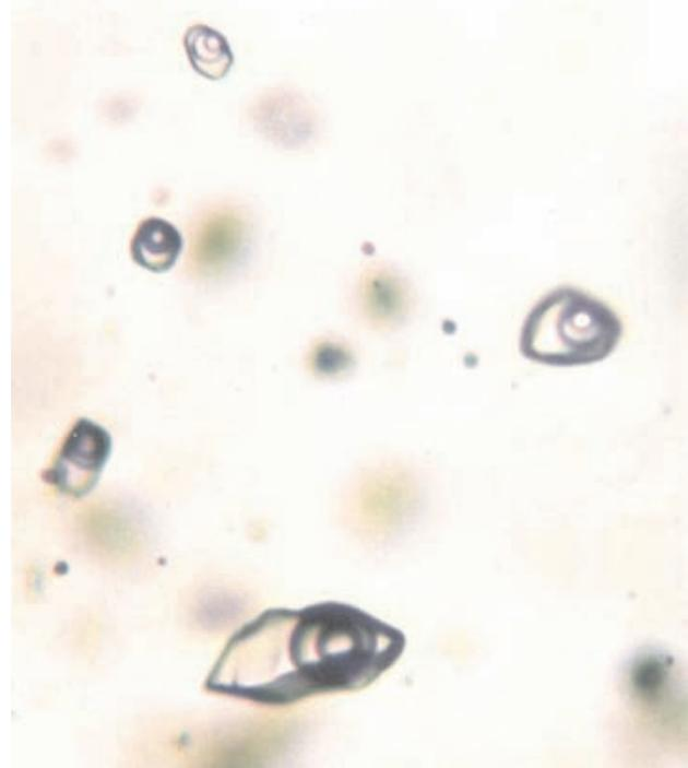
Photo 15. Smooth to negative - crystal shaped Type IV fluid inclusions in quartz from a quartz vein, Mosquito Creek deposit. Note the three  $\text{CO}_2$  and  $\text{H}_2\text{O}$  phases present at room temperature ( $20^\circ\text{C}$ ). Sample GR-00-67. Transmitted plane light. Width of photo 160  $\mu\text{m}$ .
