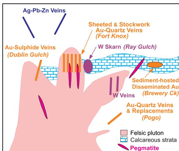
Figure 2. Schematic model of plutonic-related mineral deposits, showing different styles and zonation of intermediate to felsic “reduced” plutons intruded into a continental margin setting.
