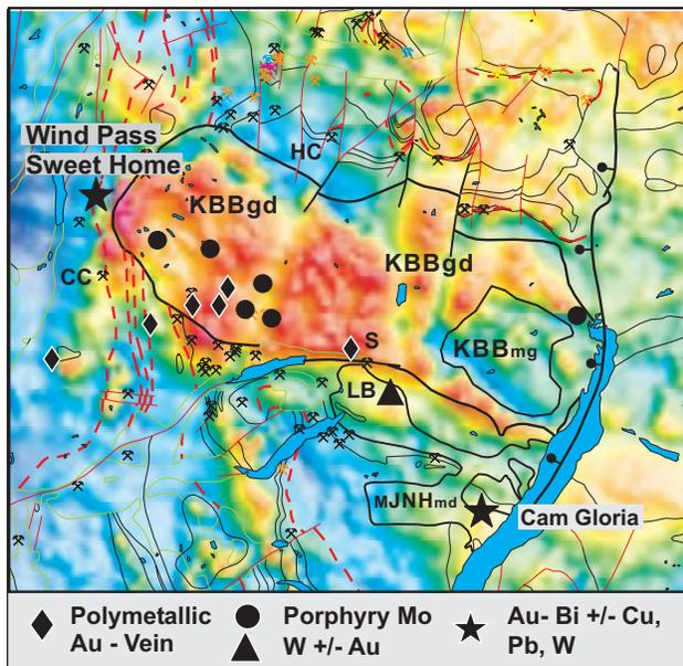
Figure 8. Aeromagnetic intensity survey map showing distribution and various styles of mineralization related to Cretaceous Baldy magmatism. The hornblende-biotite granite phase in the western 2/3rds of the batholith is distinct from the biotite-muscovite granite in the east and the hornblende quartz monzodiorite of the Honeymoon stock.
