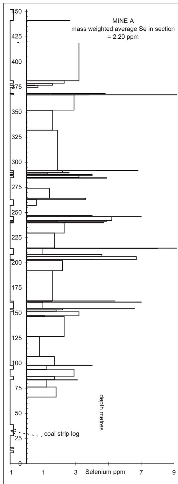
Figures 6 to 10. Stratigraphic sections at the 5 mines (A, B, C, D, and E) illustrating variation of Se content with depth. Locations of coal seams are indicated. Data below detection limit (0.2 to 0.8 ppm) are plotted as detection limit.
