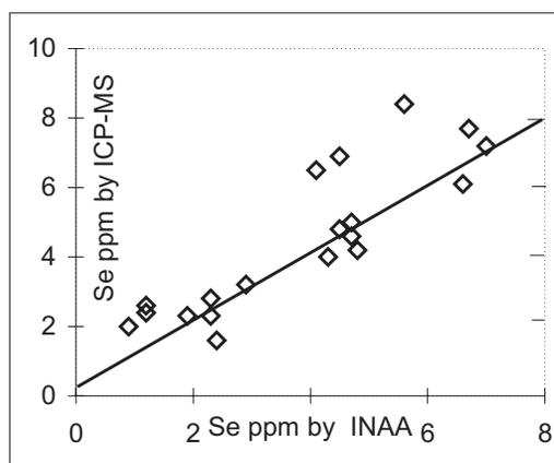
Figure 4. Cross plot of Se concentrations determined by INAA and ICP-MS.
