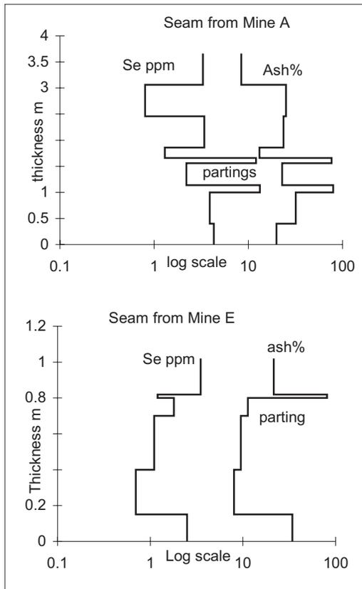
Figure 14. Se concentrations of incremental samples through 2 seams, Mines A and E.
