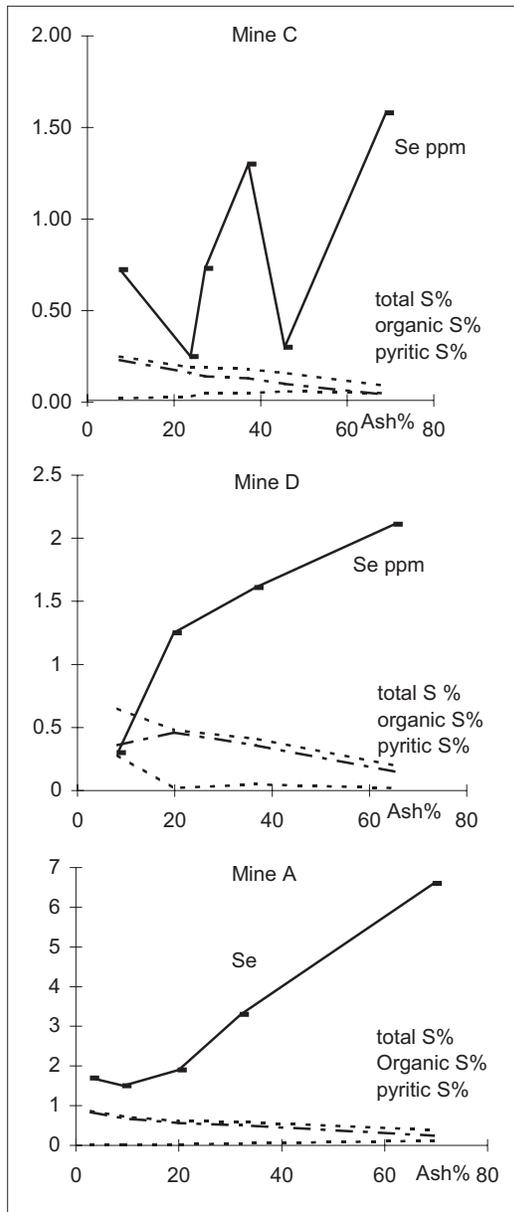
Figure 16. Se wash data for coal samples from mines C, D and E.
