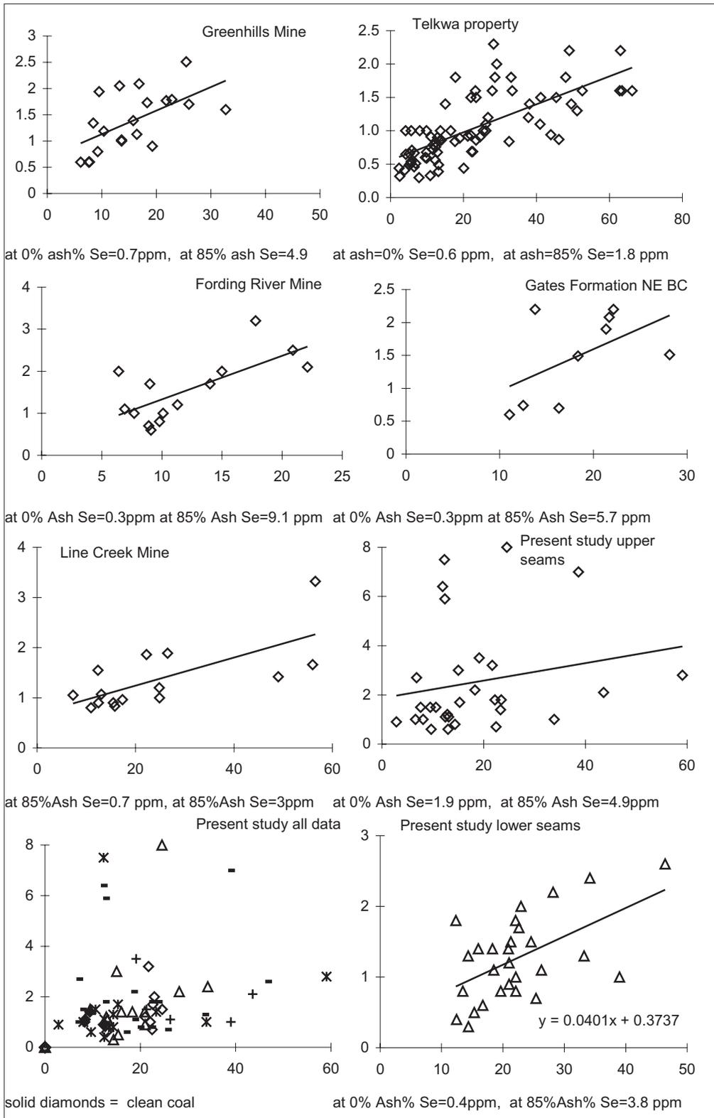
Figure 13. Ash versus Se plots for coal samples from a number of mines and properties data from this study, unpublished Geological Survey reports, Grieve and Goodarzi (1994) and Goodarzi (1988).
