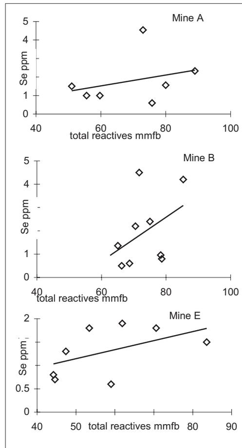
Figure 17. Average total reactives for seams from mines A, B and E versus Se content (mmfb, mineral matter free basis).
