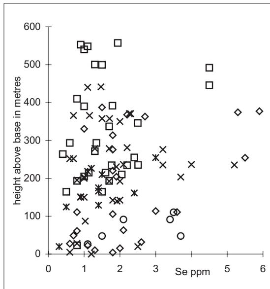
Figure 11. Se content in seams *versus* elevation above Moose Mountain Sandstone, data for all five mines; cross=mine A, square=mine B, star=mine C, circle=mine D, diamond=mine E.
