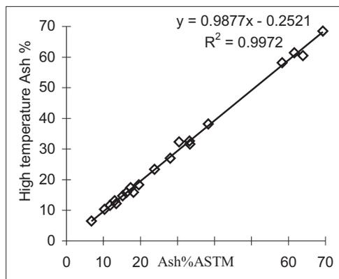
Figure 5. Cross plot of ash determined by ASTM and high temperature ashing methods.
