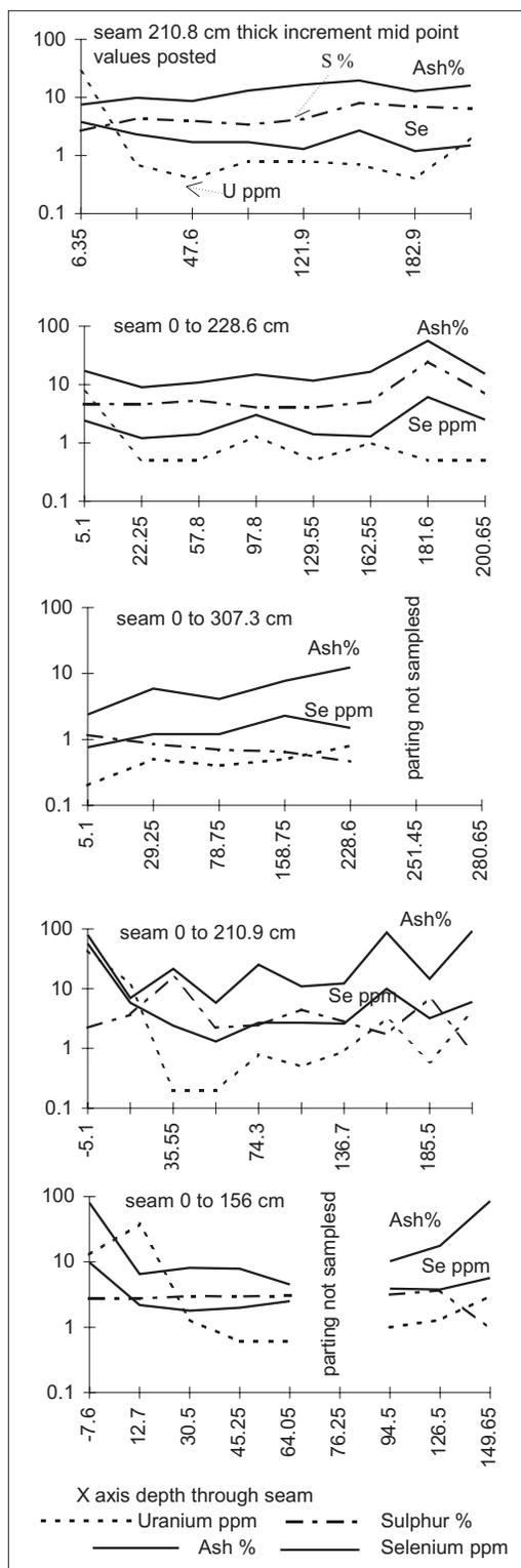
Figure 2. Se, U, S and ash in bench sample data from Gluskoter *et al.* (1977).
