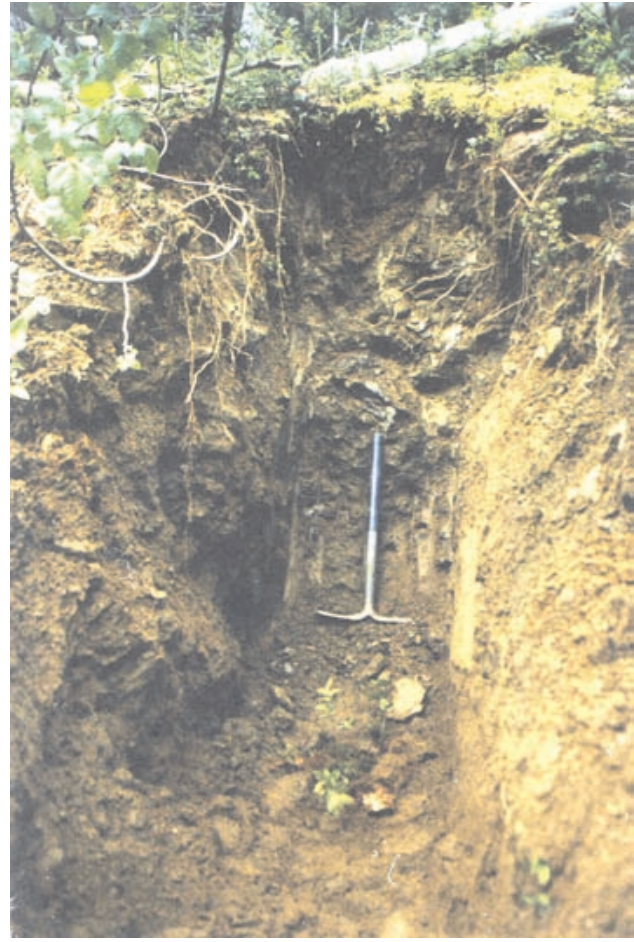
Photo 4. Till trench excavated using a small back-hoe alongside a road as part of the Ace Project. Trenches were up to a metre wide and up to three metres deep, thereby allowing for samples to be collected from various depths in the sediment profile.
