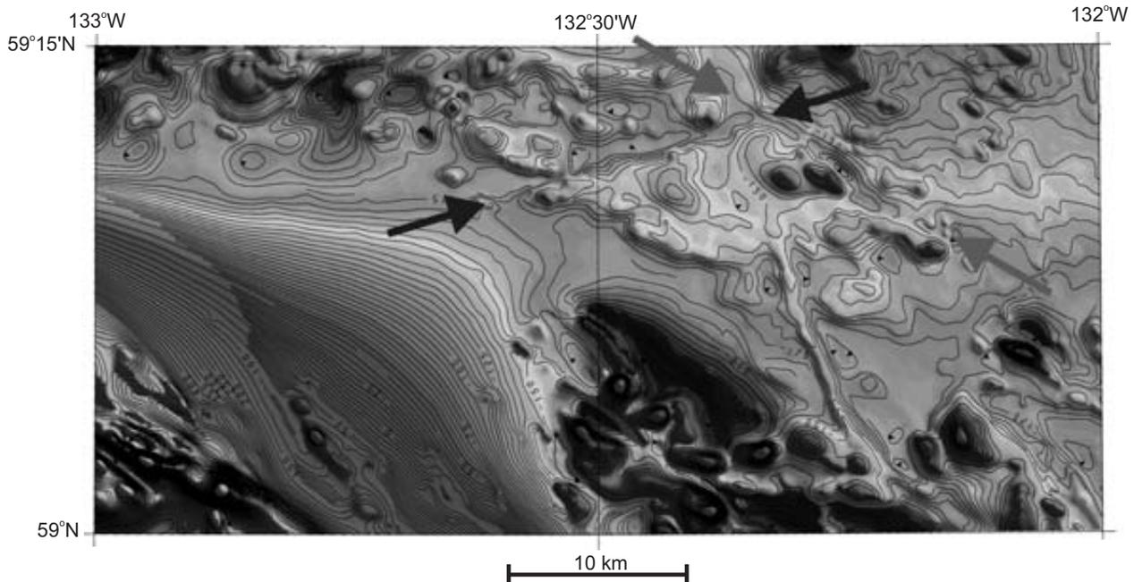
Figure 3. Aeromagnetic results for the Nakina map area, NTS 104N/1 and 2. Arrows show the location of linear negative anomalies as discussed in text. (See web page for colour version).
