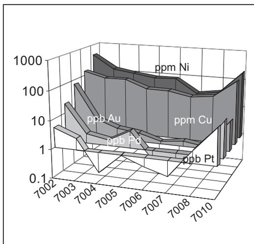
Figure 3. Elements in B-horizon soil (-80 mesh fraction) across the Sappho property.
