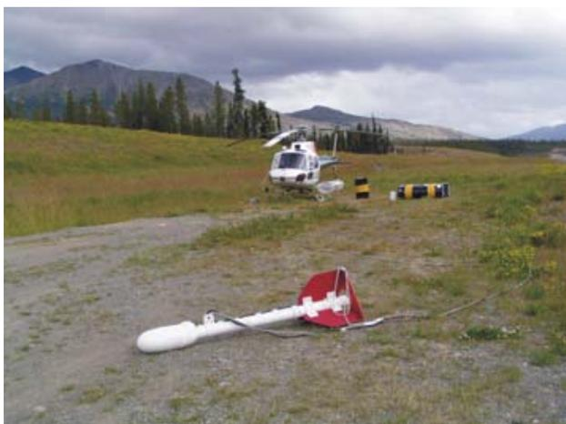
Figure 3. Cesium split-beam magnetometer is housed in a "bird" (foreground), towed 30 m below the helicopter.
