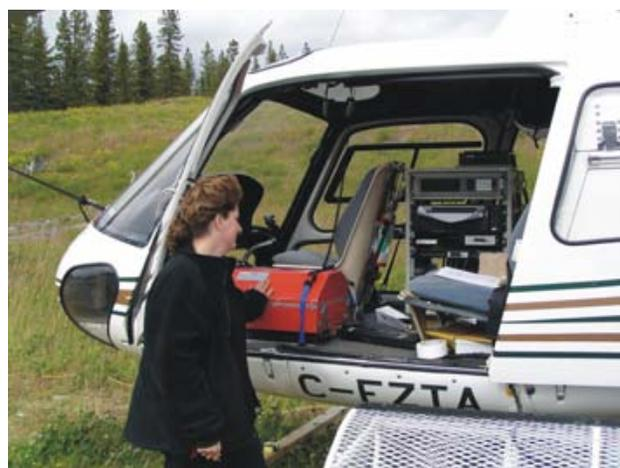
Figure 2. Gamma-ray spectrometric system includes two sodium iodide detector boxes mounted inside (orange box) and outside (in white cage, lower right) the helicopter, linked to spectrometer console in the system rack, behind pilot.
