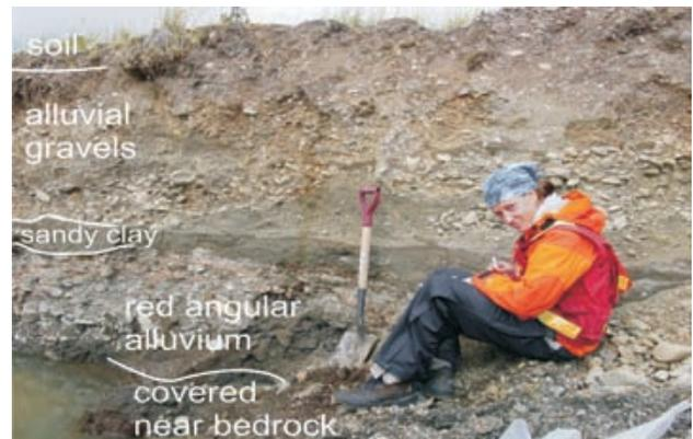
Figure 4c. Representative trench on Feather Creek showing a section of red angular alluvium, sandy clay and alluvial gravels.
