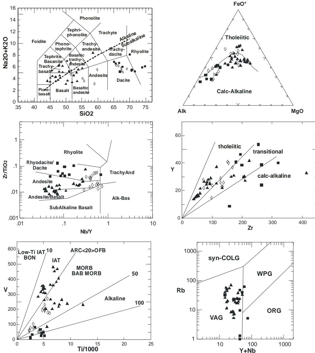
Figure 6. Geochemical discriminant diagrams for volcanic and shallow intrusive rocks in the southern Whitesail Lake study area. Closed squares indicate felsic tuffaceous and intrusive units and closed triangles indicate mafic intrusive and extrusive units. Open diamonds are analyses of felsic and mafic samples from the vicinity of the Nifty prospect (data from Ray et al., 1998).
