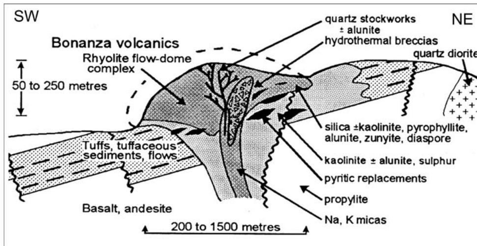
Figure 1. Schematic relationships between permeable lithologies, volcanic structures, hydrothermal conduits and mineralization in the Pemberton Hills area (Panteleyev and Koyanagi, 1993).
