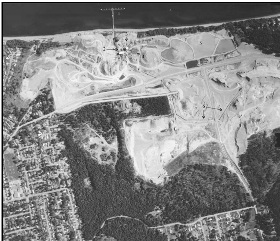
Figure 4. Aerial extent of the Metchosin gravel pit (aerial photograph PIM-C-90013 #156, scale 1:5000). 1) barge loading facility, 2) washing and screening plant, 3) aggregate stockpile area, 4) water recycling tank, 5) tailing ponds and 6) field conveyor belt system.
