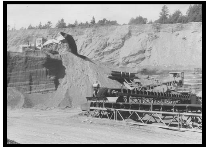
Figure 6. Front-end loader extracting gravel and dumping it into a feed hopper. This aggregate is run through a primary field crusher. Crushed aggregate is then conveyed to the processing plant for final screening.
