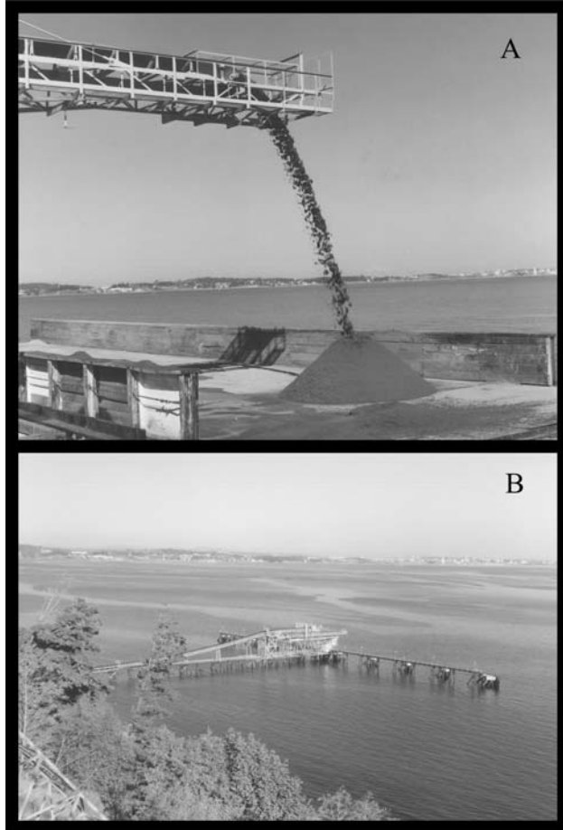
Figure 5. A) Photo showing how barges are loaded at Construction Aggregates Limited Producers Pit. B) Construction Aggregates Limited barge loading facility.
