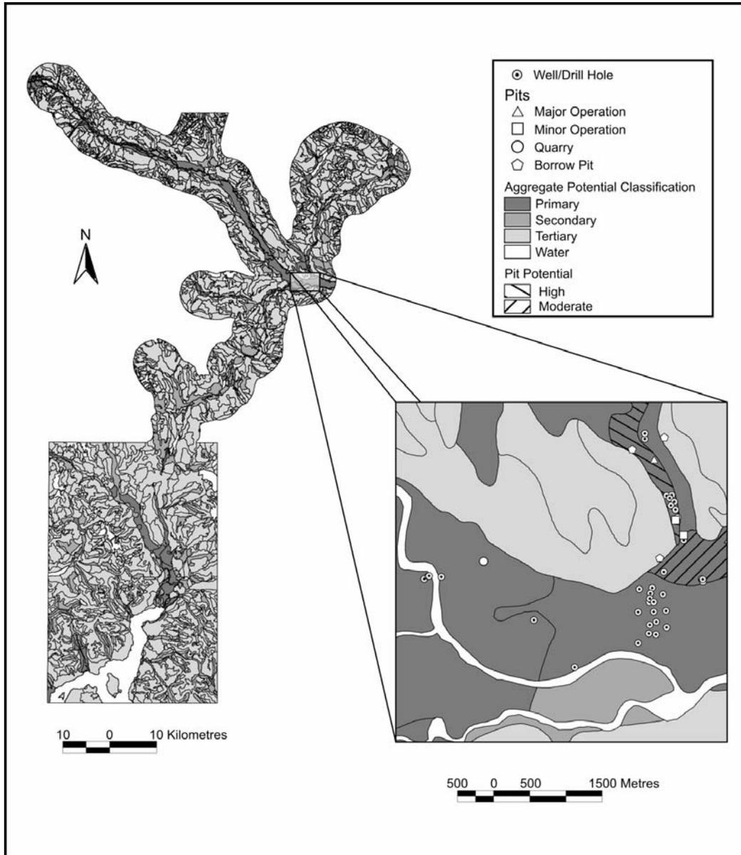
Figure 2. The final Sea-to-Sky Aggregate Potential map displays the distribution of the three polygon classes (primary, secondary, and tertiary). The insert is a magnified portion of the study area showing the additional information included in this project (Lillooet River, east of Pemberton). This information consists of drill hole and pit locations, as well as the pit potential for polygons hosting historic or active aggregate operations.
