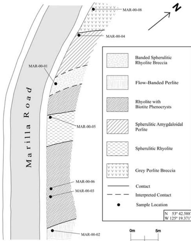
Figure 4. Outcrop at the Marilla perlite occurrence seen in plan view. It shows the six major lithological units.
