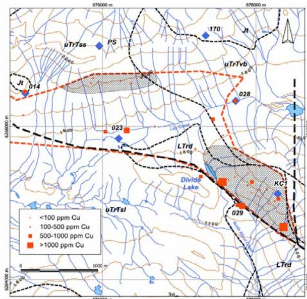
Figure 6. Copper values for samples collected in the Divide Lake area as part of the current study. See Figure 2 for legend.
