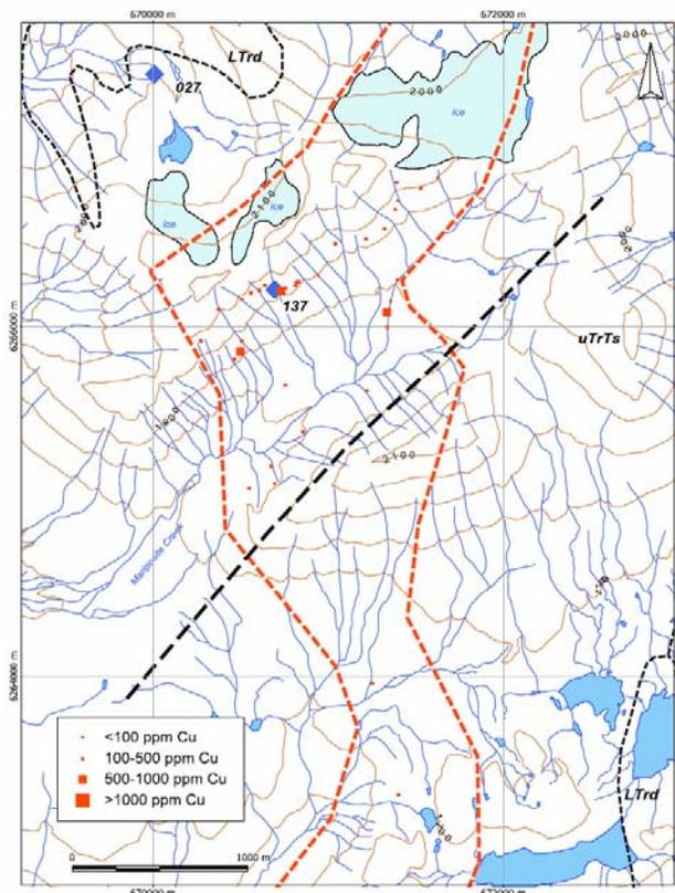
Figure 10. Copper values for samples collected in the Mariposite Creek area as part of the current study. See Figure 2 for legend.
