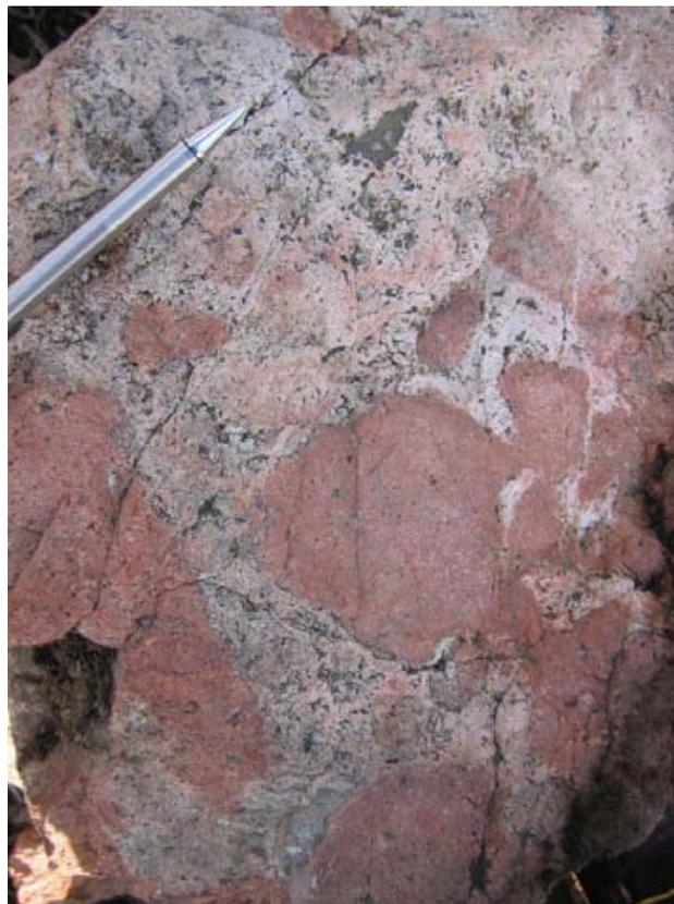
Figure 13. Intrusive breccia characterized by pervasive potassic alteration and frothy, albite replacement along clast margins. Breccia defines the western contact of the Mount Polley monzo-syenite stock located on Mount Polley.
