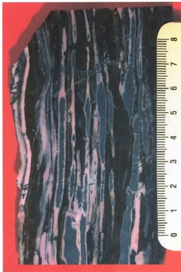
Figure 1. Sample of chert with braunite lenses and rhodonite-pyroxmangite rims.
