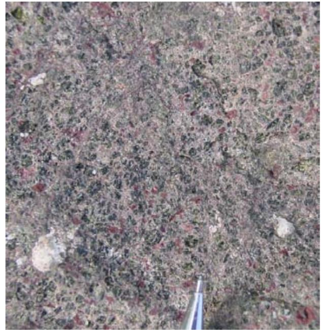
Figure 6. Typical flow, comprising euhedral pyroxene, plagioclase and olivine replaced by bright red iddingsite.
