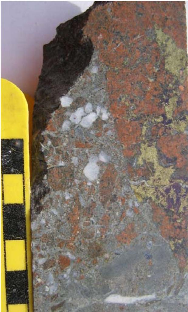
Figure 18. Post-mineral hydrothermal breccia with an albite-clinozoisite alteration overprint. Note clasts of mineralization within matrix.
