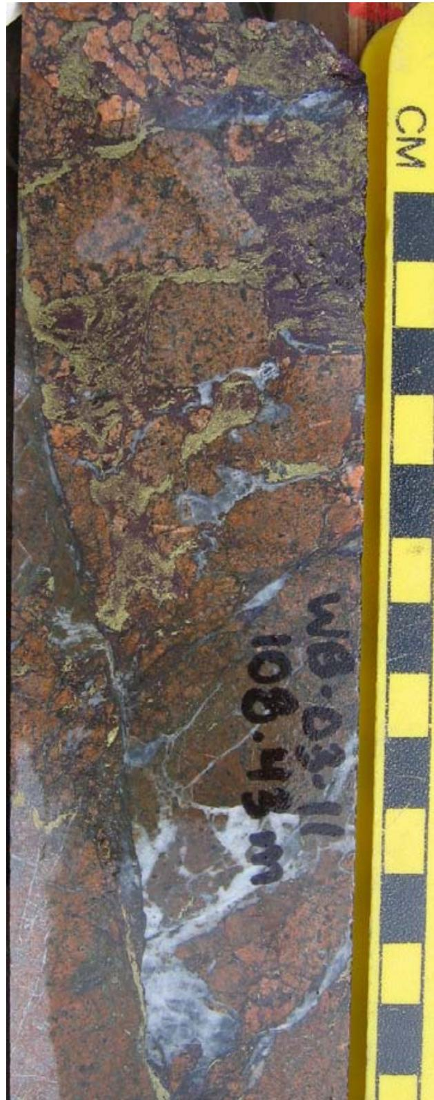
Figure 19. Coarse intergrown clots of chalcopyrite and bornite in fractures cutting potassic altered monzonite breccia in the Northeast zone.
