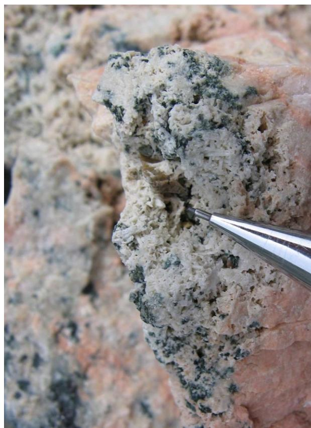
Figure 18. Vuggy intergrown matrix of K-feldspar and albite with calcite, chalcopyrite, pyrite and coarse euhedral crystals of sphene filling open spaces.
