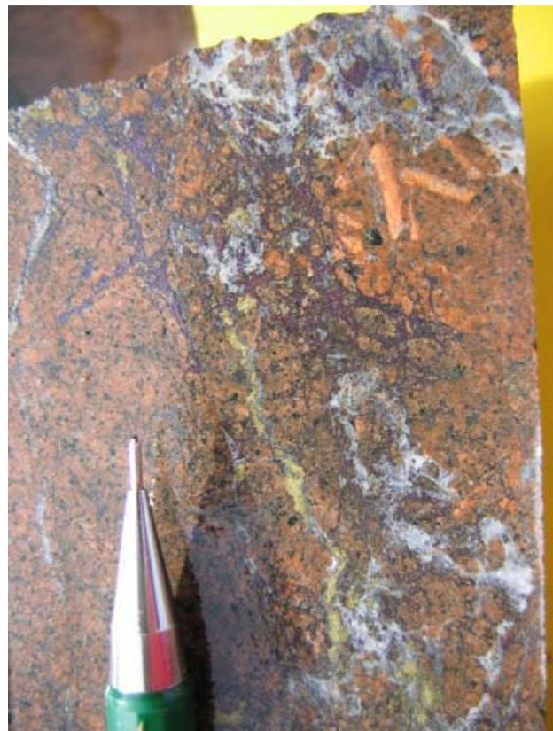
Figure 11. Mineralized fragments of K-feldspar porphyritic monzonite-syenite in breccias at the Northeast zone.
