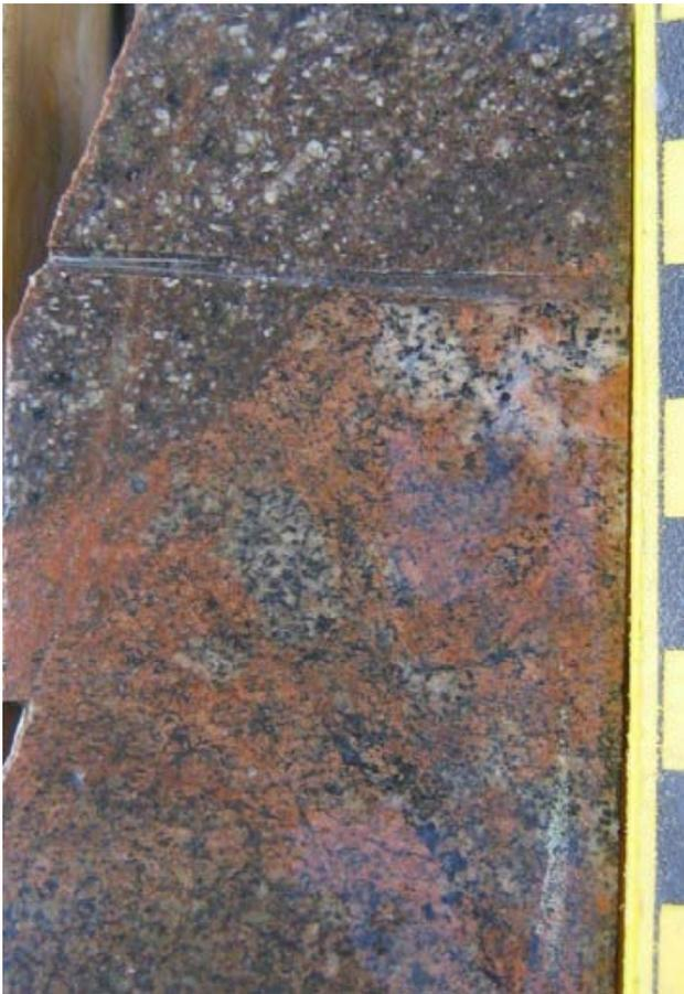
Figure 10. Plagioclase porphyry dike, chilled margin against pervasive potassium metasomatized monzodiorite. Drillcore from beneath Bell pit.
