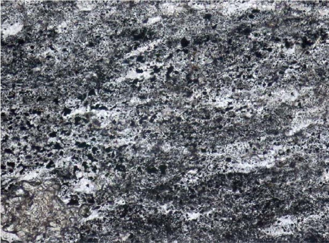
Figure 8. Photomicrograph (100x) of chert with disseminated braunite.
