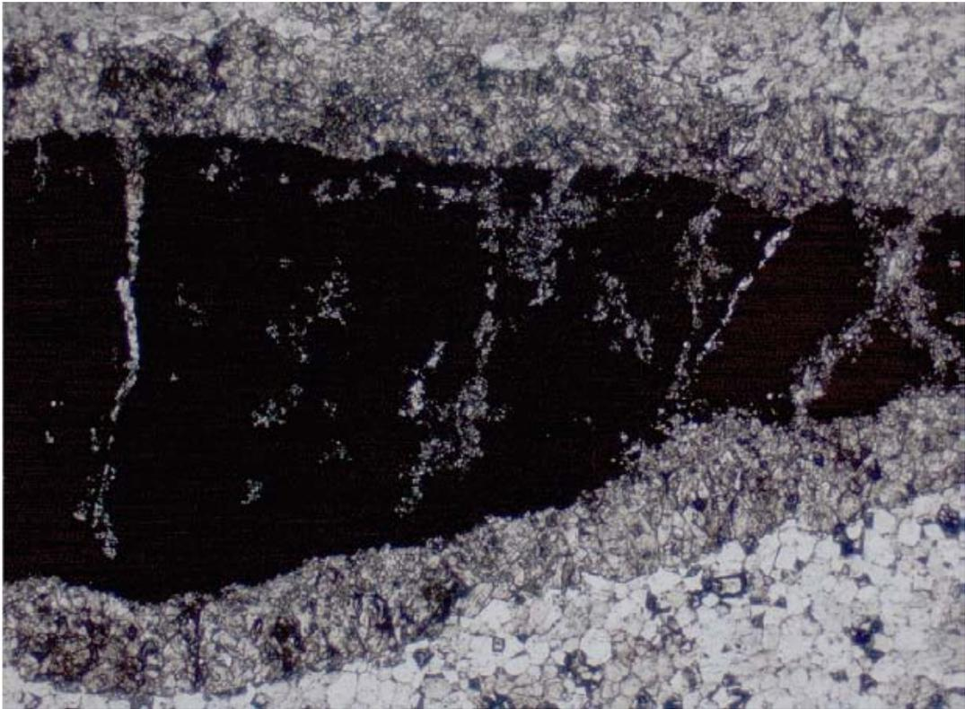
Figure 2. Photomicrograph (25x) of braunite lens with Mn-silicate rim in chert.
