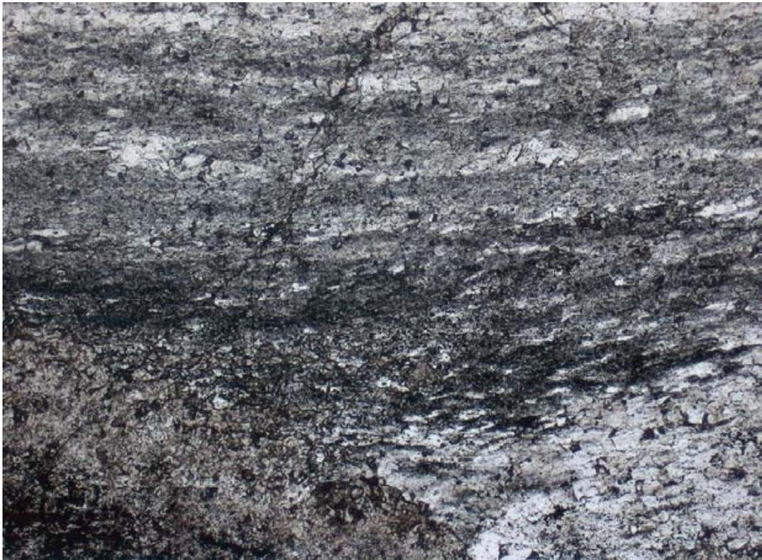
Figure 6. Photomicrograph (25x) of chert with disseminated braunite.
