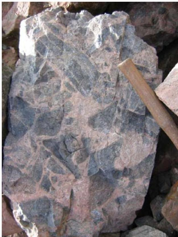
Figure 12. Intrusion breccia, plagioclase porphyry in the Cariboo pit
