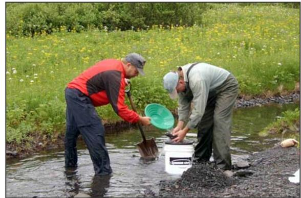
Plate 1. Bulk stream sediment sample collection.
