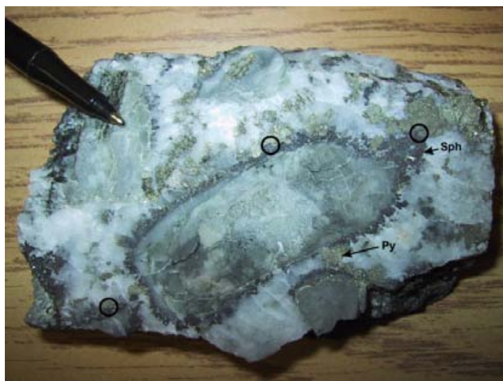
Figure 10. Slab of quartz carbonate vein containing brecciated vein material rimmed by sphalerite (Sph) and pyrite (Py). The circles indicate the areas where coexisting pyrite and sphalerite were sampled for sulphur isotopes. Pen for scale.
