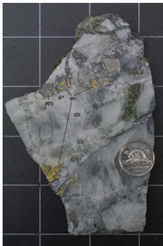
Figure 5. Slab of gold-bearing quartz (qtz) vein from the Privateer mine. Slab length is approximately 15 cm. Note the relationship between the galena (gn), which replaces arsenopyrite (apy), and the gold (au), which cuts both arsenopyrite and galena.
