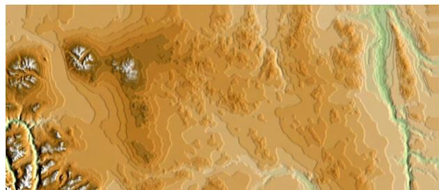
Figure 3. Digital elevation model for map sheets 093B (east half of figure) and C (west), derived from 20 m contour elevation data generalized to 100 m. Fraser River (east margin), Chilcotin River (south centre) and the three peralkaline Anahim Belt volcanoes of the Igachuz Range are prominent. Note steps in elevation model are emphasized in low-relief areas. Far Mountain is on the north side of the middle Anahim Belt volcano.
