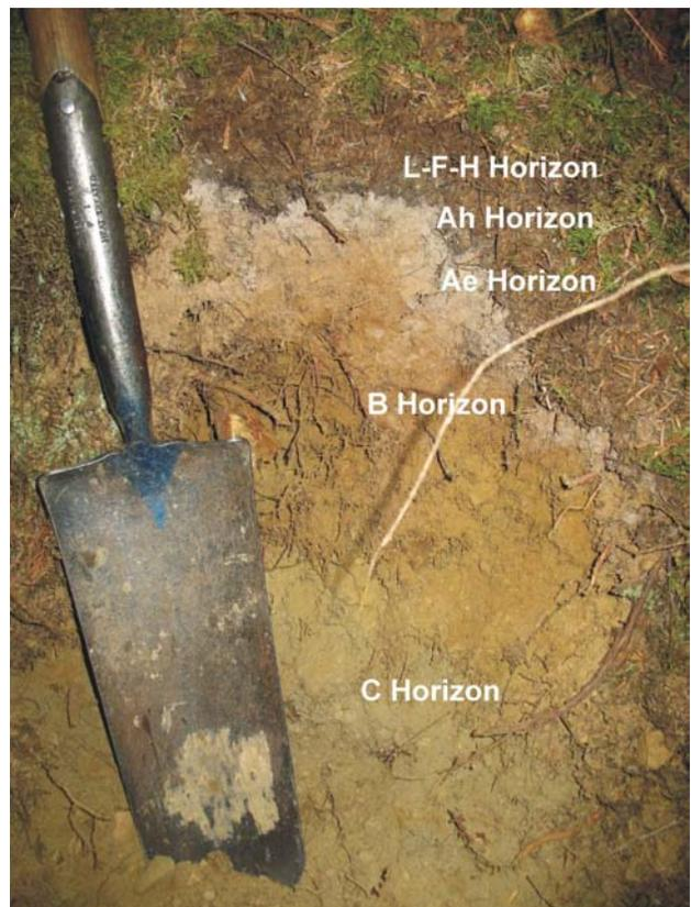
Figure 2. Profile showing Brunisolic soil developed on till, Mouse Mountain area.
