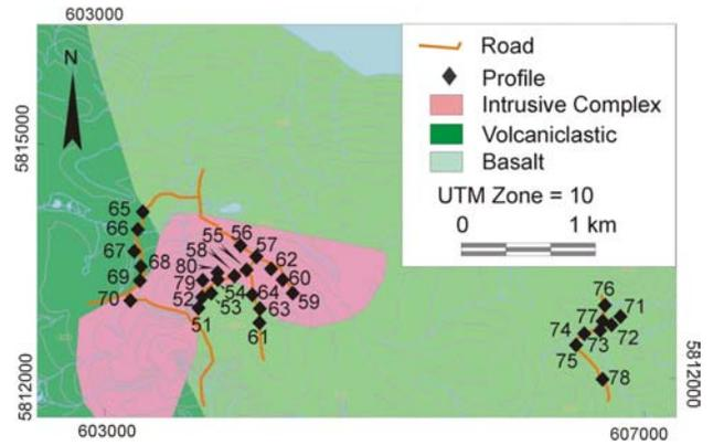
Figure 9. Soil profile locations over the Shiko Lake property (geology after Massey et al., 2005).
