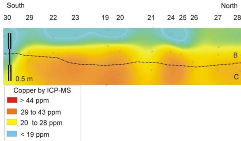
Figure 13. Contoured Cu in soil along a north-south traverse, Yorston and Coyote lakes (Soda Creek) area.
