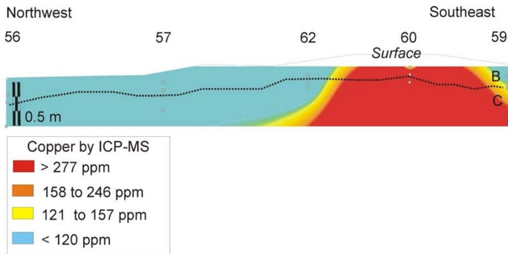
Figure 10. Contoured Cu in soil between profiles 56 and 59, Shiko Lake.
