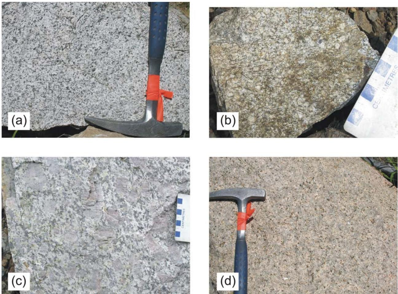
Figure 12. Intrusions of the Beaverdell area. a) hornblende-biotite granodiorite of the Jurassic Westkettle batholith (07NMA28-20; UTM Zone 11, 5484322N, 360440E, NAD83); b) hornblende crowded feldspar diorite (07NMA34-13; UTM Zone 11, 5474088N, 359662E, NAD83); c) typical K-feldspar megacrystic granite of the Eocene Coryell suite (07NMA45-09; UTM Zone 11, 5475024N, 355570E, NAD83); d) pink quartz monzonite of the Eocene Coryell suite (07NMA28-17; UTM Zone 11, 5486026N, 360995E, NAD83).
