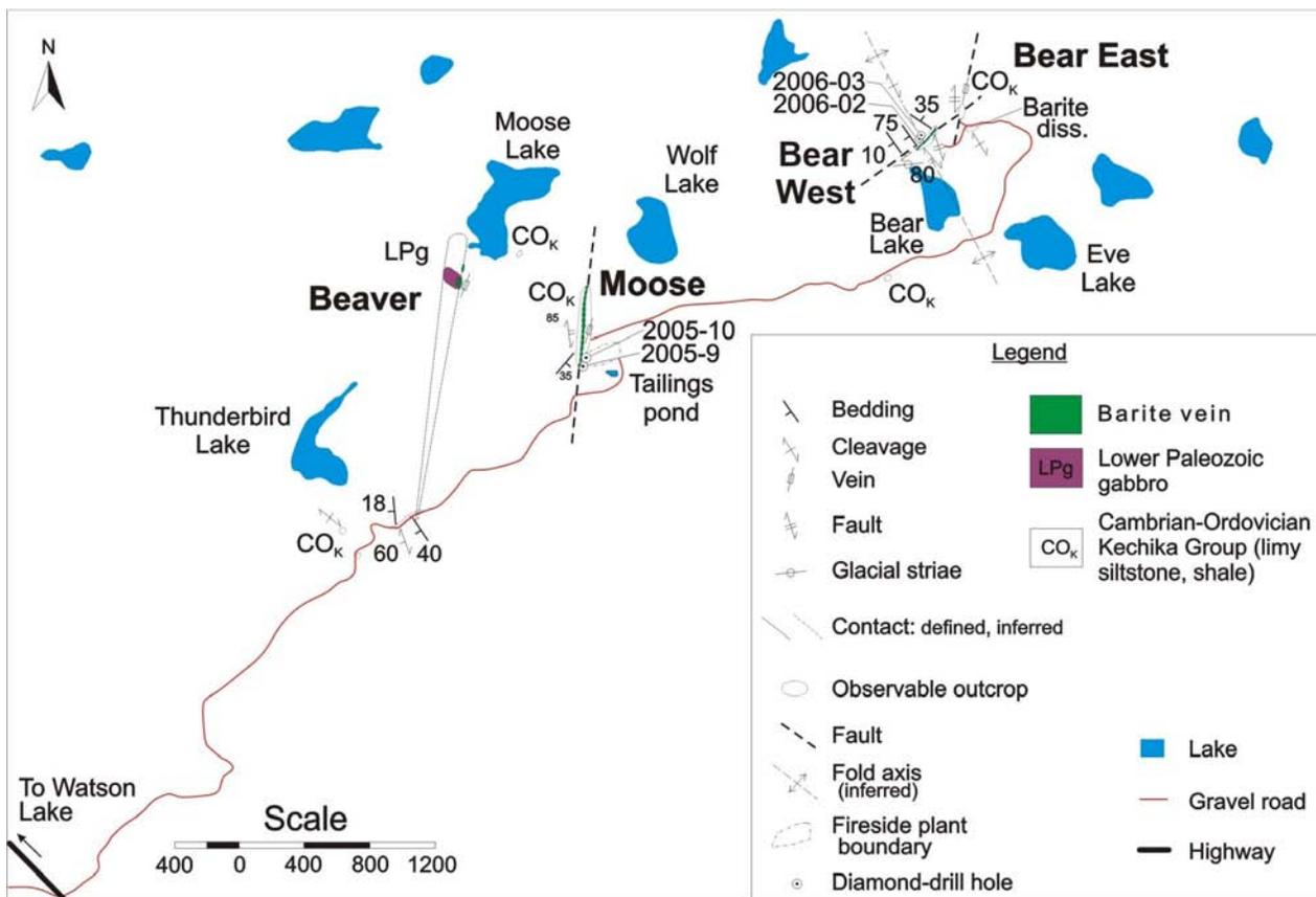
Figure 5. Geology of the Fireside barite minesite.
