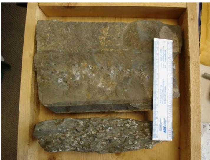
Figure 7. Barite crystals in siltstone.
