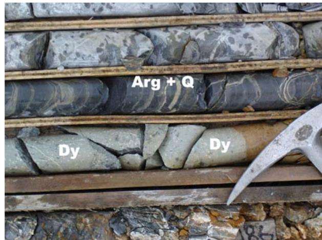
Figure 11. Altered mafic dike (D) and veined argillite (A) in diamond-drill hole 2005-09.
