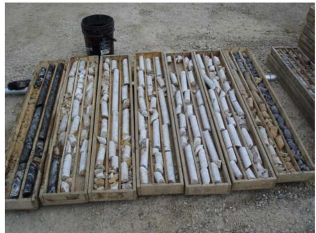
Figure 10. Barite vein intercept below the Bear West pit in diamond-drill hole 2006-02; black footwall breccia is also visible.
