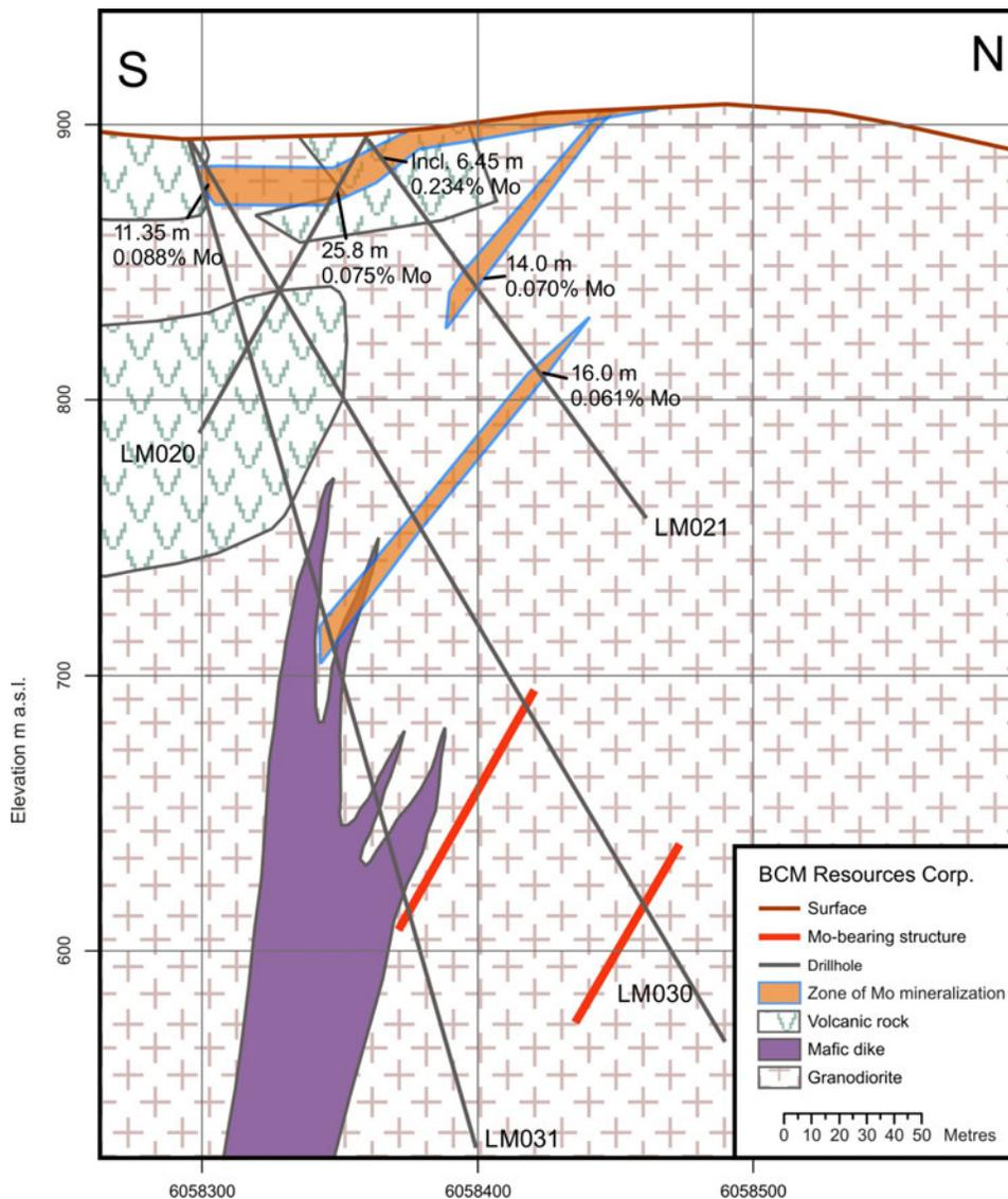
**Figure 7.** Section 536350 E, Shan South property (see Figure 4 for location). Note that zones of Mo mineralization are zones with significant visible Mo mineralization that should be tested with additional drillholes, and include intercepts with 0.06% Mo cutoff, as quoted in press releases (BCM Resources Corp., 2007).
