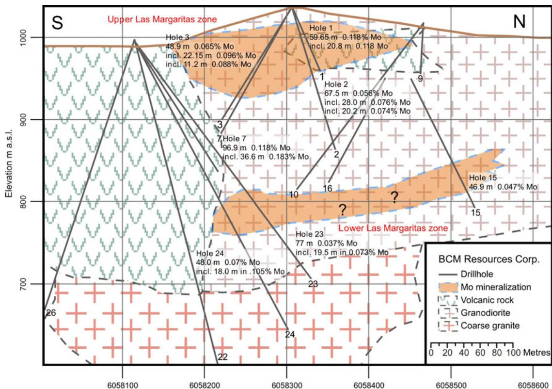
**Figure 5.** Section 535800 E through the Upper and Lower Las Margaritas zones, Shan South property (see Figure 4 for location). Note that zones of Mo mineralization are zones with significant visible Mo mineralization that should be tested with additional drillholes, and include intercepts with 0.06% Mo cutoff, as quoted in press releases (BCM Resources Corp., 2007).
