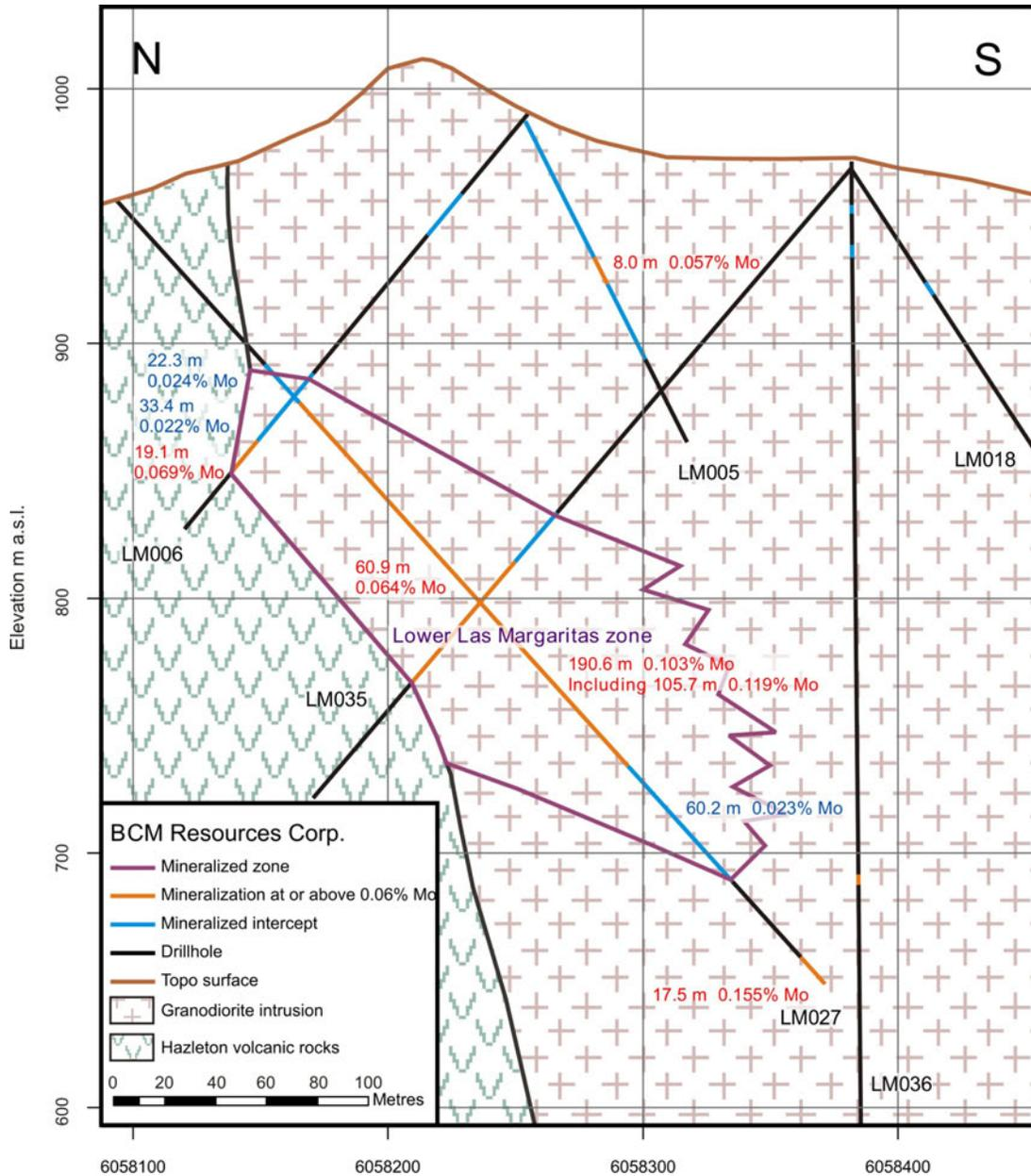
**Figure 6.** Section 536000 E through the Lower Las Margaritas zone, Shan South property (see Figure 4 for location). Note that zones of Mo mineralization are zones with significant visible Mo mineralization that should be tested with additional drillholes, and include intercepts with 0.06% Mo cutoff, as quoted in press releases (BCM Resources Corp., 2007).
