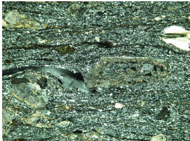
**Figure 14.** Photomicrograph of mylonite zone in Middle Jurassic K-feldspar-megacrystic monzogranite of the Quesnel River pluton (3 mm field of view; crossed polars).
