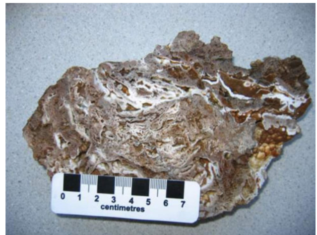
Figure 11. Cut through a hemimorphite nodule from Oxide deposit, south-eastern British Columbia, displaying characteristic texture.
