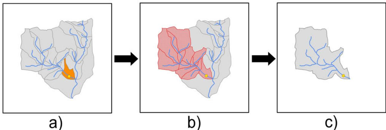
Figure 3. Catchment basin delineation stages depicted with examples: **a)** locate root watershed (highlighted in orange) for a sample site (yellow dot), **b)** retrieve all upstream watersheds (highlighted in red) and **c)** dissolve the upstream watersheds as the catchment basin for the sample site.
