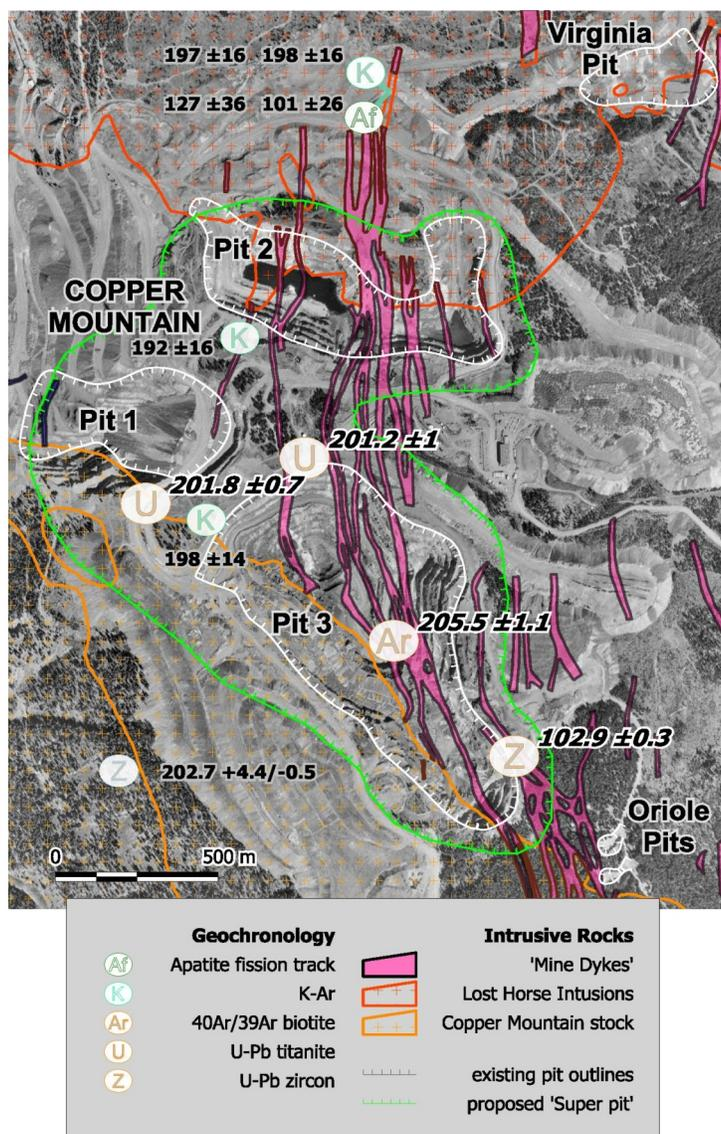
**Figure 3.** Locations of geochronological samples collected as part of this study (large symbols) and those collected previously by other authors (smaller symbols) as reported in the database compiled by Breitsprecher and Mortensen (2004), Copper Mountain area, south-central British Columbia. Geological contacts and underlying imagery are adapted from Preto et al. (2004). The proposed ‘super pit’ outline is from Chance et al. (2009). Values on the map are in Ma.
