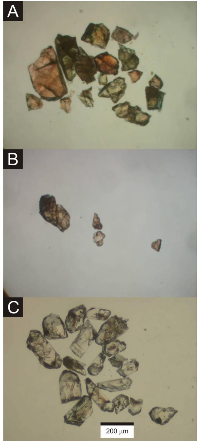
**Figure 7.** Titanite grains analyzed from samples from Copper Mountain, south-central British Columbia: **A)** titanite from sample MMI06-32-3; field of view is  $\sim 2$  mm; **B)** titanite from sample MMI06-32-5; field of view is  $\sim 2$  mm; **C)** zircon separate from sample MMI06-32-4 prior to abrasion (200  $\mu$ m scale bar).
