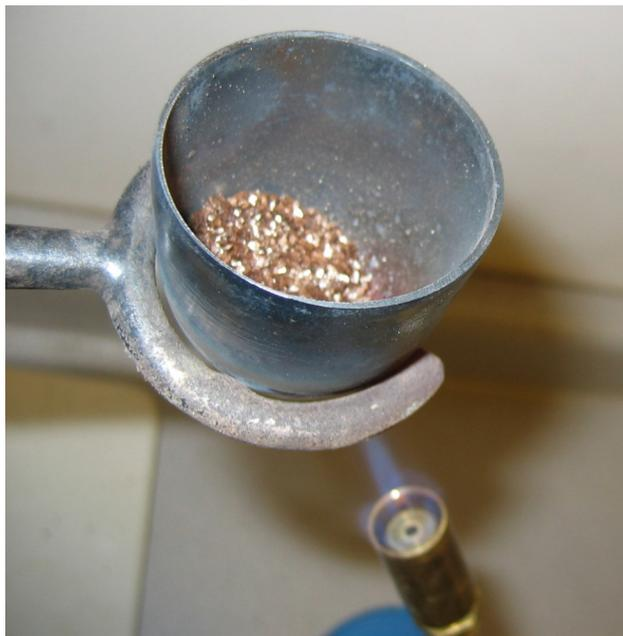
**Figure 7.** Crude laboratory set-up used to exfoliate vermiculite-bearing rock samples taken from the outcrop adjacent to the Hodgje rare earth zone, Blue River area, east-central British Columbia.
