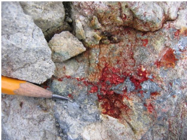
**Figure 5.** Typical bright red stain caused by reaction of “Zinc Zap” solution with zinc-rich mineralization, east-central British Columbia.
