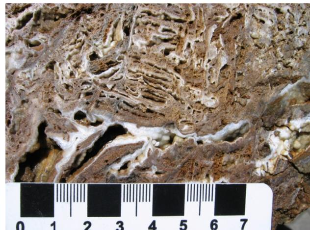
Figure 3. Hemimorphite-rich mineralization, Oxide deposit, southeastern British Columbia. The hemimorphite replaced the carbonate groundmass.
