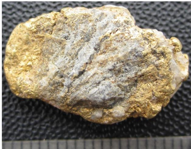
**Figure 6.** Nugget from Snake Creek is gold intergrown with rock which is like thermally-altered argillaceous chert comprising the bedrock upstream. Scale divisions are millimetres.
