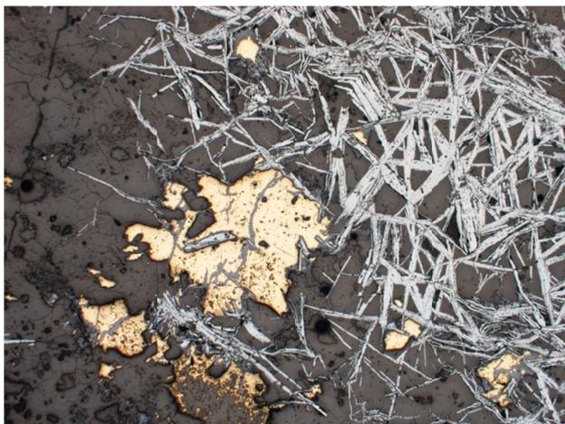
**Figure 22a.** Skarn mineralization at the Birthday Jim occurrence: photomicrograph of reflected light view of bladed specular hematite which is enclosed by late chalcopyrite. Accessory pyrite occurs outside the ~5 mm field of view.
