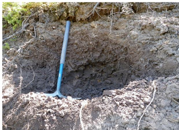
**Figure 5.** Clayey silt to silt rich, overconsolidated diamicton, interpreted as a basal till. Well developed vertical jointing and subhorizontal fissility give this basal till a blocky appearance. Pick for scale (65 cm).
