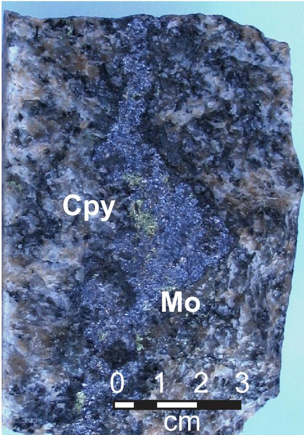
**Figure 5.** High-grade molybdenite (Mo) – chalcopyrite (Cpy) mineralized fracture cutting weakly altered hornblende quartz granodiorite of Takomkane batholith. Drill core from Southeast zone, drillhole WJ07-79.
