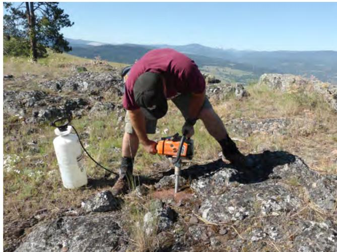
**Fig. 5.** Drilling an oriented core for paleomagnetic study at Miner Mountain in the Nicola Arc-South project area.
