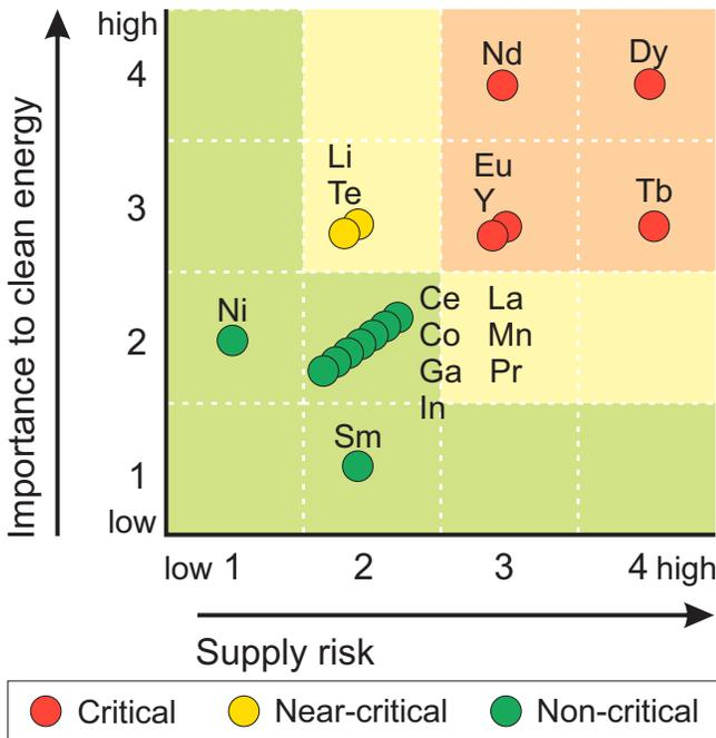
**Fig. 3.** US Department of Energy criticality matrix of 16 elements for 2015-2025, based on importance to clean energy and supply risk. Modified from US Department of Energy (2011).
