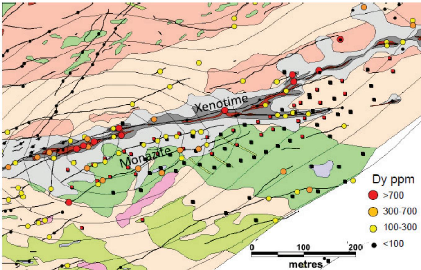
**Fig. 3.** Distribution of dysprosium in surface samples of the potential ore zone on the Lofdal property. The dark grey denotes a zone of intensely fenitized Huab gneisses adjacent to a fault; the surrounding light grey area is a zone of weaker fenitization. The other lithological units are: amphibolite (green); calc-silicate gneiss (apple green); granitic gneiss (light pink); quartzofeldspathic gneiss (tan) and pegmatite (pink).
