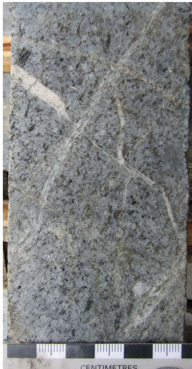
Fig. 4. Ragged hornblende quartz diorite porphyry, a mineralized intrusive phase in DDH SH028 at the Dick Creek zone, sampled for U-Pb-zircon SHRIMP geochronology (sample 14ZE920A).
