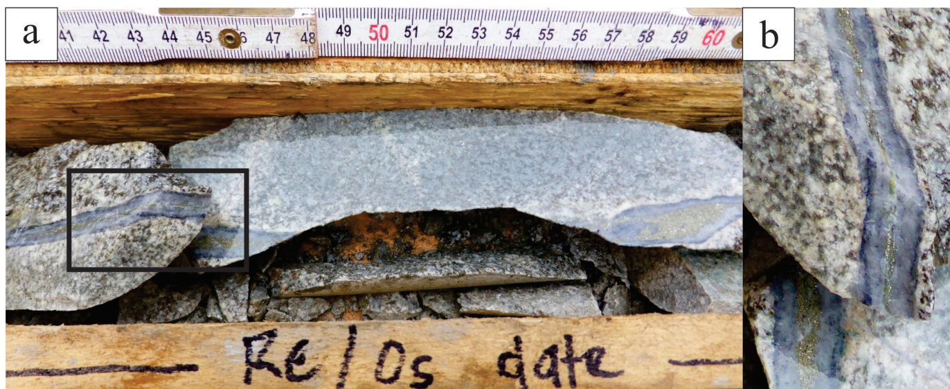
Fig. 5. a) Drill core of altered quartz diorite cut by stockworks of quartz-pyrite-molybdenite \pm chalcopyrite-epidote-chlorite veinlets and veins up to \sim 1.5 cm wide. Indicated on the core box is the segment of the core collected for molybdenite extraction and Re-Os age determination (DDH S040, 89.7-90.3m). b) Close up of a) with blue-grey molybdenite concentrated along vein margins.
