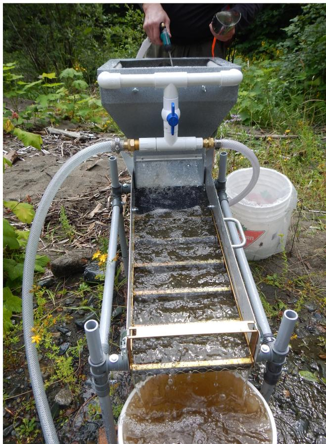
**Fig. 5.** A sluice box (25.5 cm wide) coupled with shower sample feeder set up on a stream bank.
