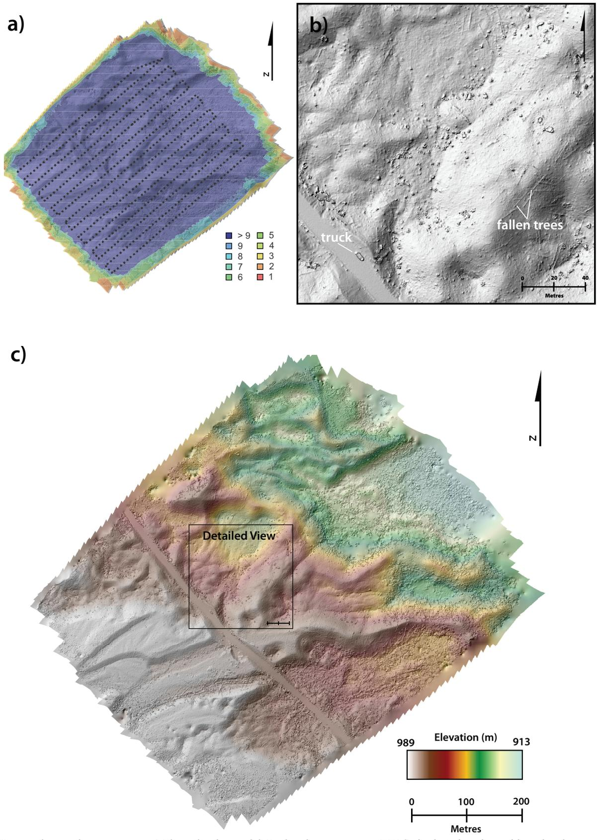
**Fig. 6.** Hummocky terrain survey area. **a)** Photo density model. Each point represents a RPAS air photo location, with each colour representing the number of overlapping photos used to create the photogrammetric DEM. See Figure 1 for location. **b)** Detailed view of survey area. Fallen trees are represented by linear, criss-crossing objects. **c)** Photogrammetric DEM of ice contact and channelized glaciofluvial sediments.
