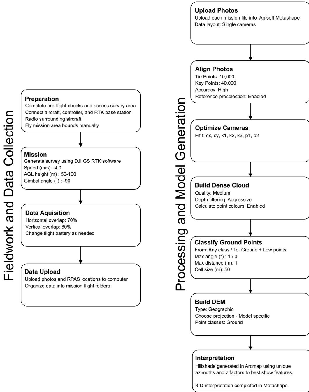
Fig. 3. Flight and data workflow for typical generation of photogrammetric DEMs.
