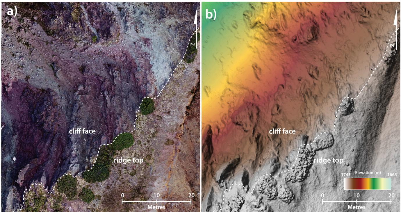
**Fig. 9. a)** Orthomosaic of bedrock ridge created from RPAS-acquired air photos. It is possible to identify and differentiate oxidized maroon rhyolites and reduced buff-white rhyolites on the northwestern cliff face. This orthomosaic is high-resolution (~3 cm/pixel) and can be used as a base map for fine-scale geologic mapping. **b)** Photogrammetric DEM produced for the same region. For general location see Figure 1, for specific location and perspective, see Figure 4.
