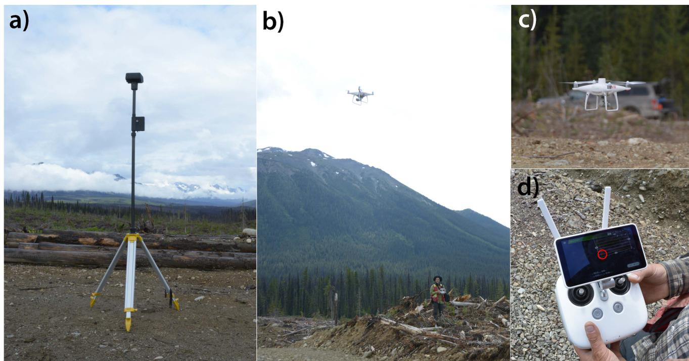
**Fig. 2.** Equipment used in the field that makes up the RPAS. **a)** RTK mobile base station. **b)** DJI Phantom 4 Pro RTK being operated remotely by pilot on-ground. **c)** DJI Phantom 4 Pro RTK in flight with the camera facing away from the viewer. **d)** DJI Remote control, with DJI flight-planning software DJI GS RTK on screen, showing location of RPAS (red circle) while conducting an air photo mission autonomously in auto pilot mode following pre-planned flight lines.
