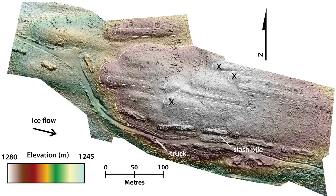
**Fig. 8.** Photogrammetric DEM of glacially streamlined terrain created from RPAS-acquired air photos. Outlined crag and tail features indicate ice flow towards the east-southeast. Bedrock outcrops represented by xs. See Figure 1 for location.
