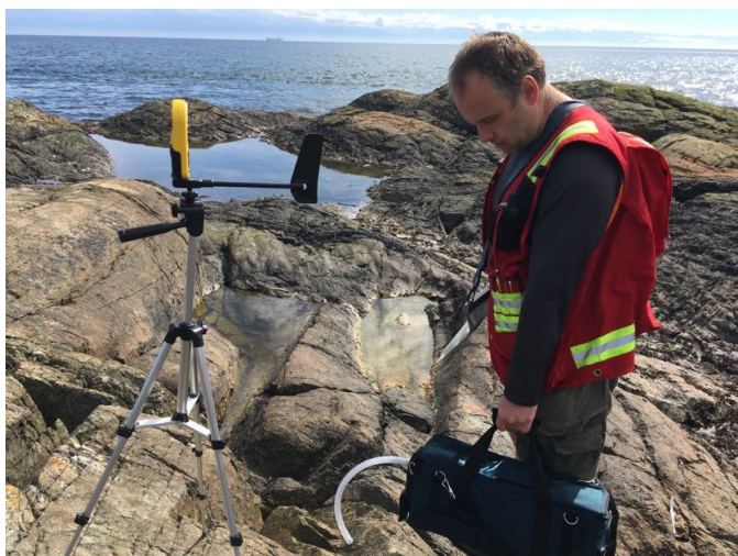
Fig. 11. Simultaneous measurement of meteorological conditions (on tripod) and direct measurement of atmospheric Hg vapour concentrations using a portable RA-915M analyzer along a terrane boundary at Harling Point, Municipality of Oak Bay, Victoria; see Rukhlov et al. (2020b, 2021b).
