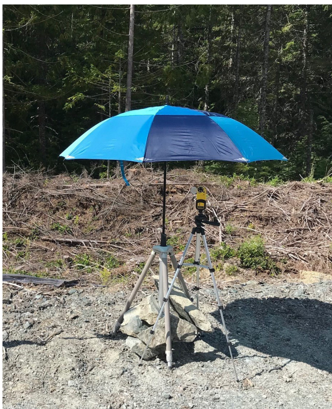
Fig. 7. Measuring air temperature, barometric pressure, relative humidity, wind speed, and wind direction (azimuth) simultaneously with the GEM concentrations.
