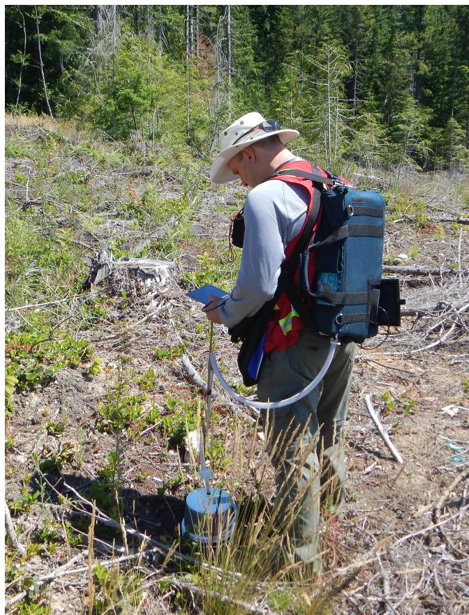
Fig. 2. Measuring real-time gaseous elemental mercury (GEM) in air 1 cm above ground.
