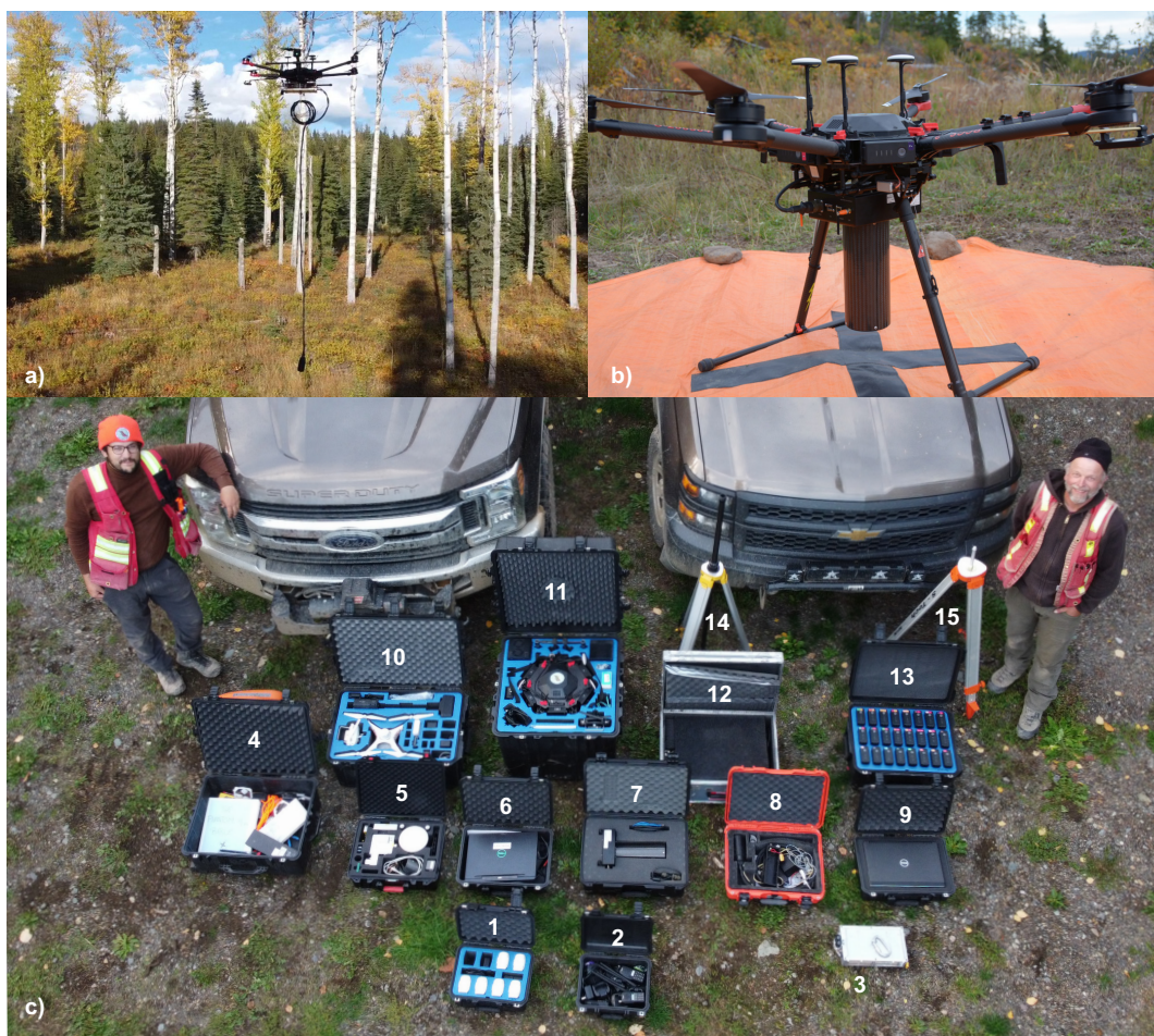
Fig. 13. a) A GEM Systems DRONEmag potassium magnetometer tethered 2.5 m below a DJI Matrice 600 Pro flying a gridded autopilot survey 7.5 m above ground level. b) A Radiation Solutions Incorporated RS-350 Backpack gamma-ray spectrometer, incorporating a 3"x3" NaI (Tl) crystal, retrofitted to a DJI Matrice 600 Pro. c) The hardware used to complete the geophysical, lidar, and photogrammetric surveys: 1. DJI Phantom 4 RTK batteries, 2. air-band handheld VHF radios, 3. magnetometer mount for DJI Matrice 600, 4. tools, VFR navigation charts, and manuals, 5. GreenValley International LiAir V70 lidar and base station, 6. laptop running GreenValley International LIDAR360 and LiAcquire software, 7. Radiation Solutions Incorporated gamma-ray spectrometer, 8. GEM Systems DRONEmag magnetometer, 9. laptop running SPH Engineering UgCS flight planning software, 10. DJI Phantom 4 RTK and base station, 11. DJI Matrice 600 Pro, 12. GSM19-G walking (base station) magnetometer, 13. DJI Matrice 600 Pro batteries, 14. RTK base station tripod, and 15. lidar base station tripod.
