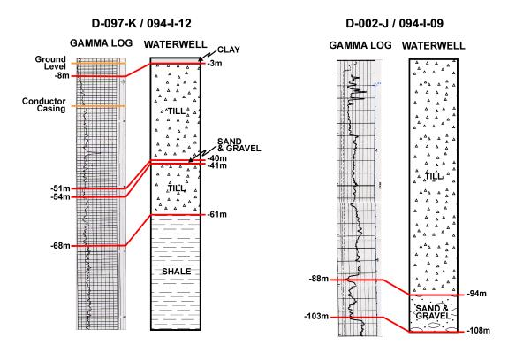
Figure 8. Examples of water well logs and nearby oil and gas well geophysical logs used in the identification and mapping of Quaternary stratigraphy, subsurface aggregates, bedrock topography and paleochannels.
