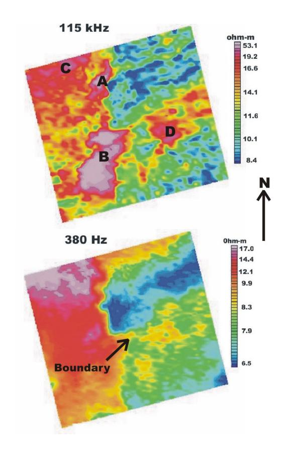
Figure 5. Apparent resistivity maps for frequencies of  $\,115\,kHz$  (upper diagram) and  $\,380\,Hz$  (lower diagram) . The four resistivity areas discussed in the text are labeled A to D in the upper diagram.
