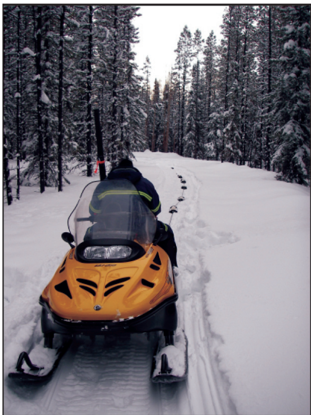
Figure 7. CCR Survey using OhmMapper™ instrument from Geometric. Five dipole-dipole receivers and a transmitter are towed behind a snowmobile.
