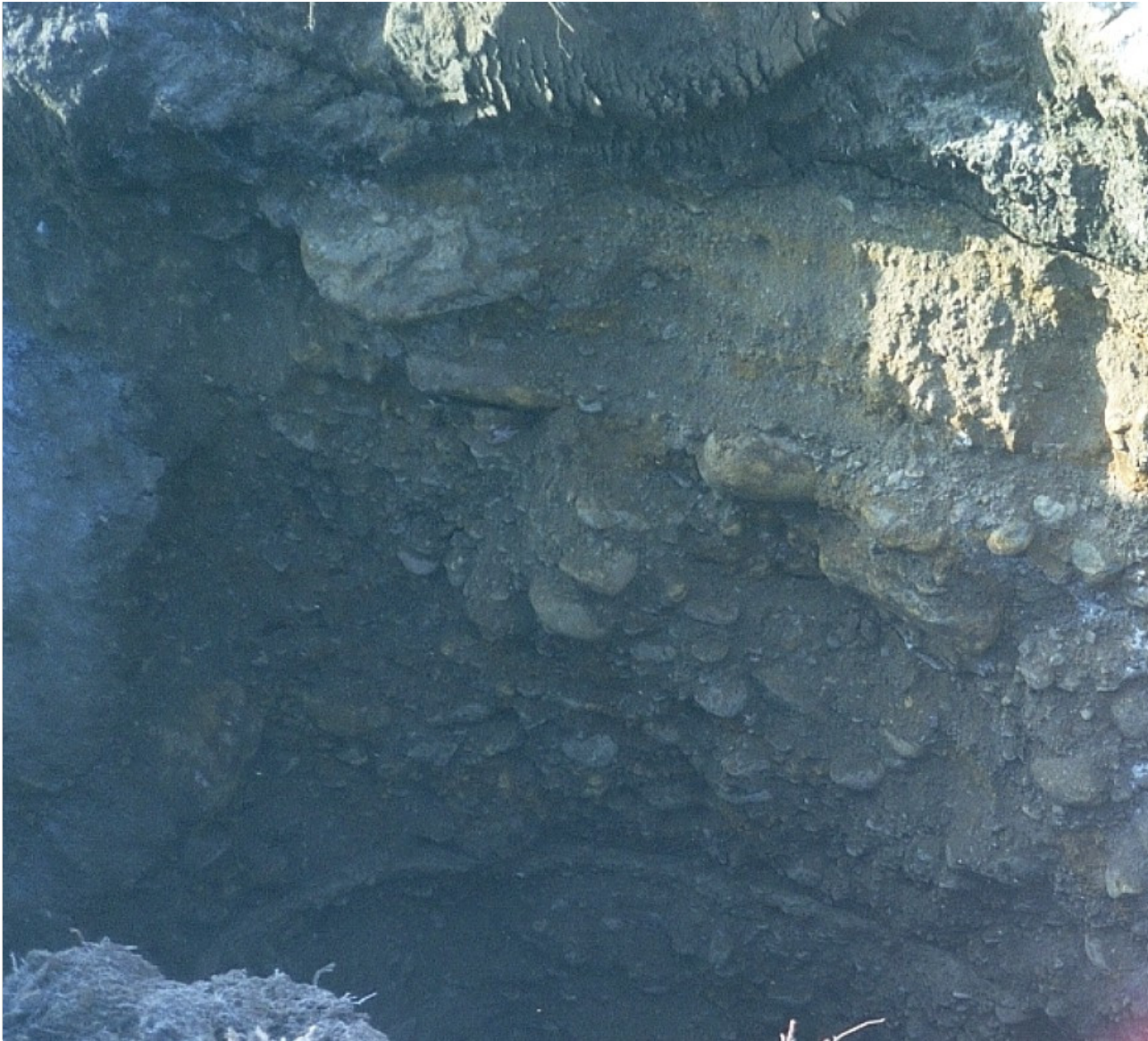
Figure 6. Test pit exposure of sands and gravels in the Kotcho East deposit buried by surficial silts. Test pit is approximately 1.5 m wide.
