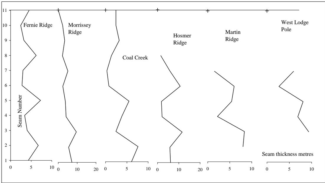
Figure 7. Plot of seam thicknesses by seam number
