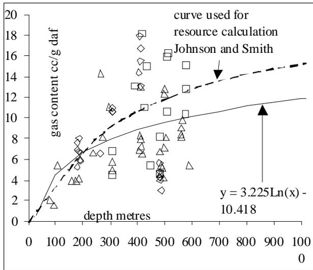
Figure 4. Desorption data Crowsnest Coalfield. Squares are for hole C12L, diamonds from Mobile Chevron holes and triangles from Saskoil holes.
