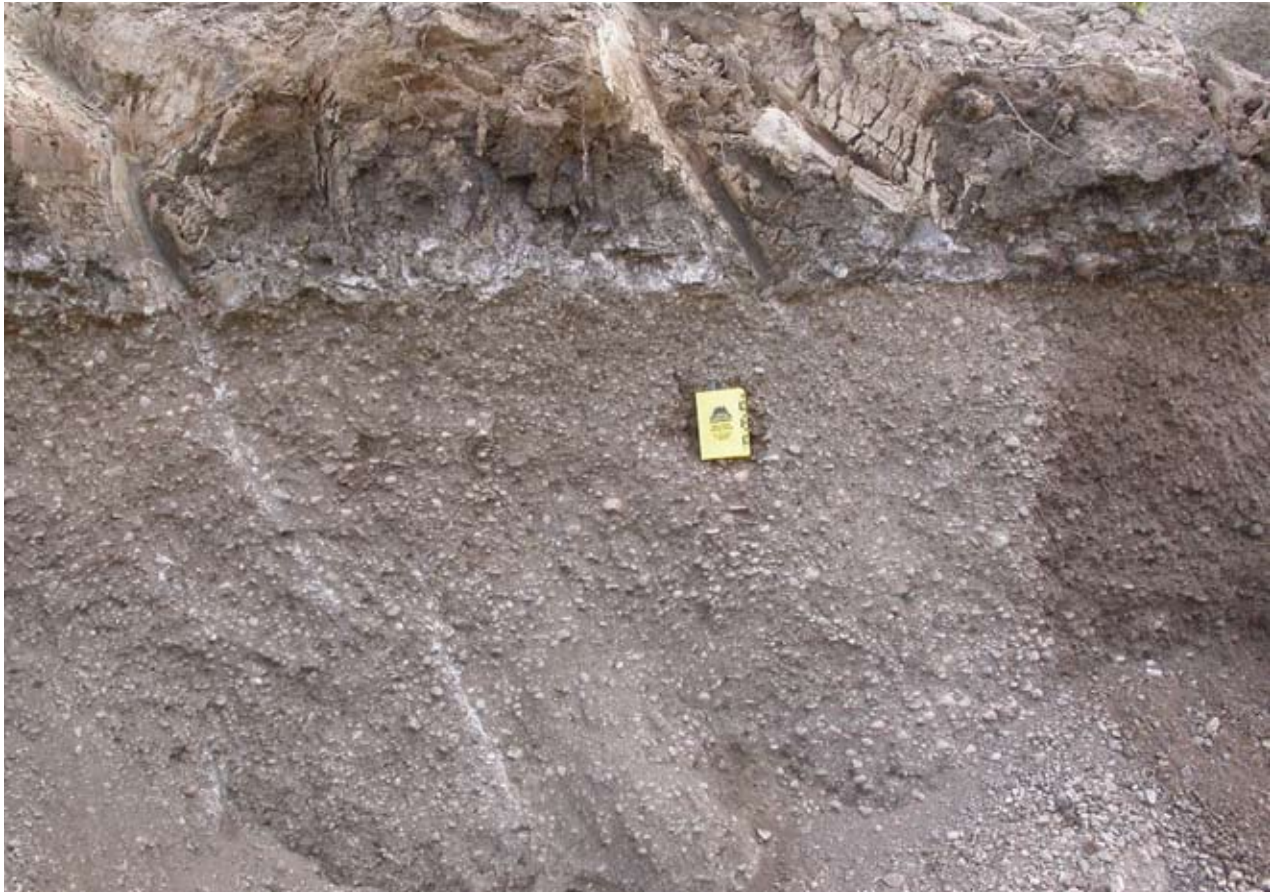
Figure 2. Sands and gravels in the Nogah Road area, interpreted to be subglacial channel deposits, underlying thin, stony, meltout till. The gravels overlie thick, clay-rich, basal till at most locations.
