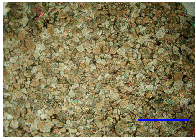
Figure 14. Photomicrographs of the Chinchaga Formation dolomites from well B-89-E/94-J-15, 8040 ft. CPL, scale bar 0.5 mm.
