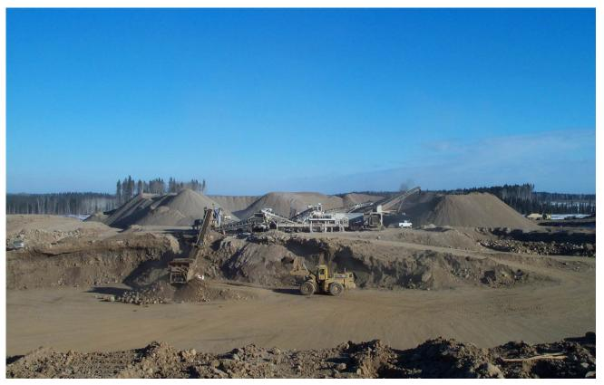
Figure 2. Active gravel mining operation during the winter of 2004 at the Elleh deposit. Aggregate from the operation was stock piled at various locations for use on the SYD and Clarke Lake Bypass roads. Gravels in the area are extensive and include mainly glaciofluvial gravels deposited during the last glaciation. (Photo provided by Quentin Huillery, Ledcor CMI Ltd.)
