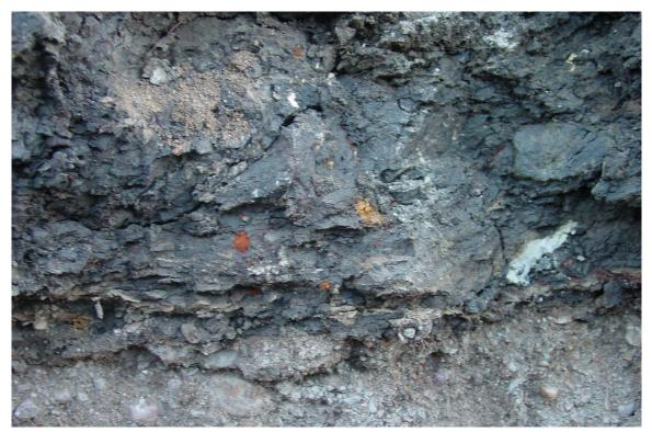
Figure 5. Close-up photo of the contact between gravels and the overlying diamict at the Kotcho East gravel pit. Note the white friable siltstone clast (about 5 cm long) in the diamict at right side of the photo. The diamict is interpreted as a basal meltout till (see text).
